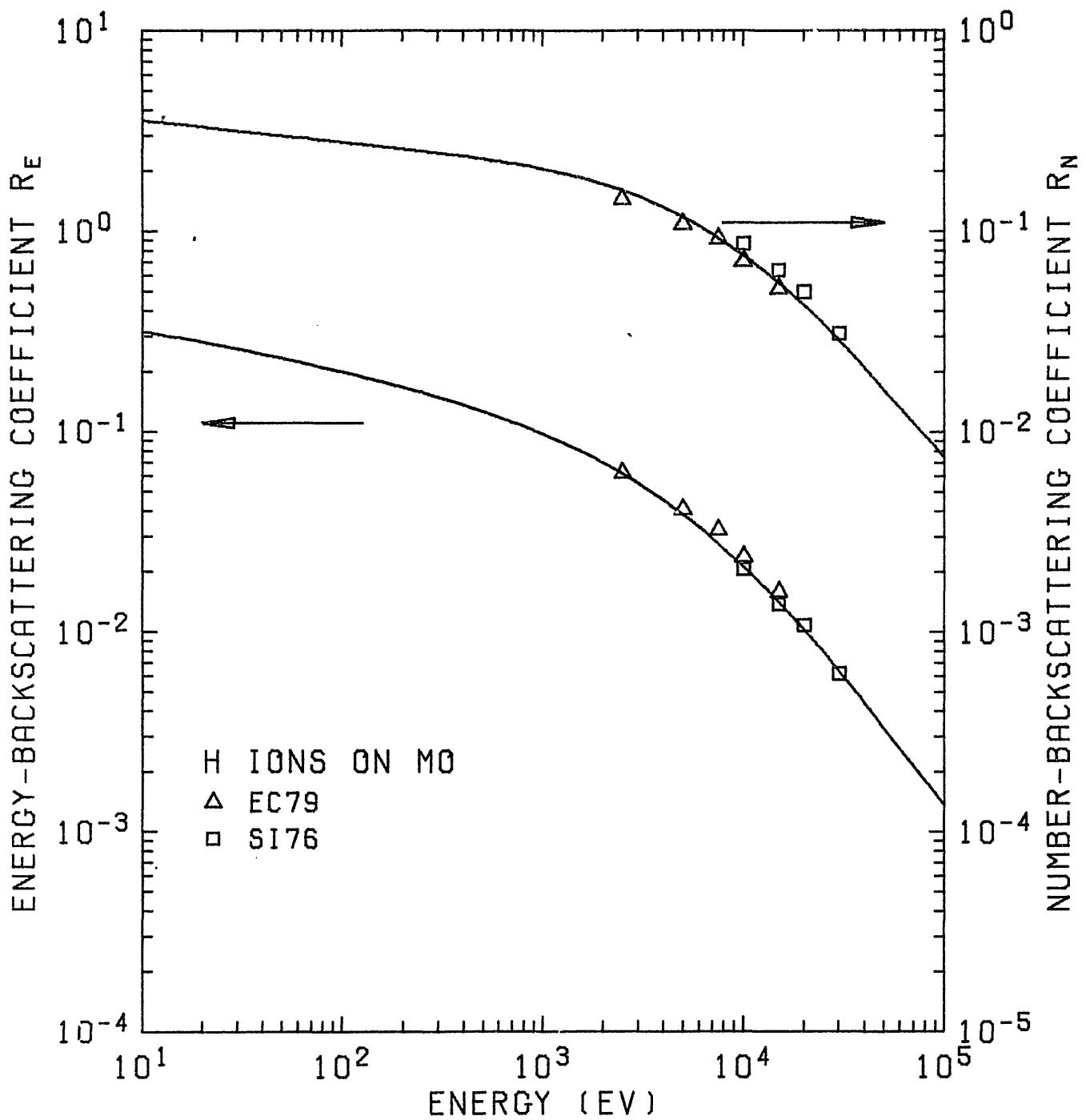
Fig. 10.  $R_N$  and  $R_E$  of H ions on  $^{42}\text{Mo}$ .
