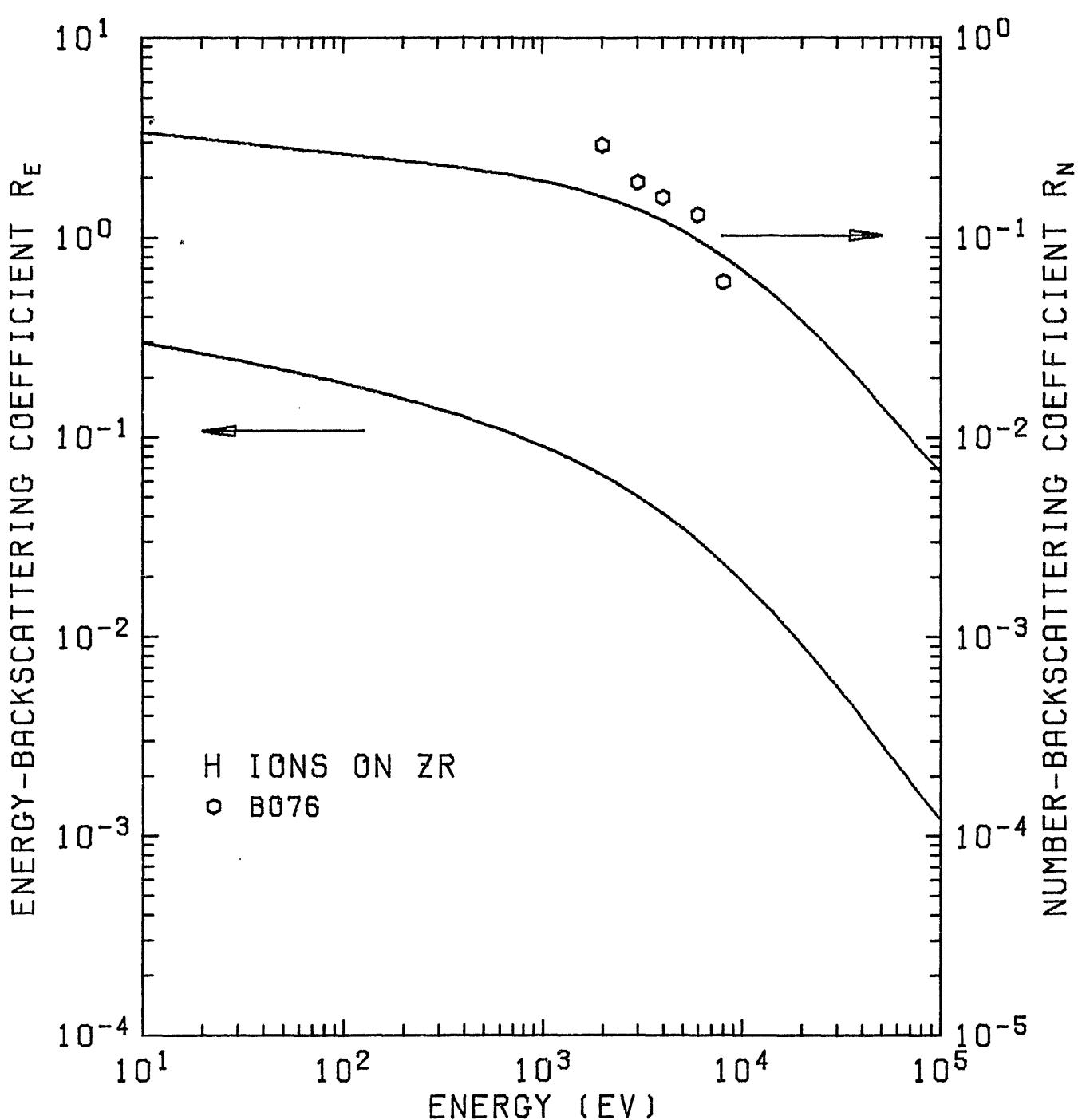
Fig. 8.  $R_N$  and  $R_E$  of H ions on  $^{40}\text{Zr}$ .
