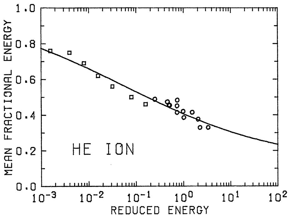
Fig. II.6. The mean fractional energy  $r_E$  of backscattered particles when He ions are incident is plotted as a function of the Thomas-Fermi reduced energy  $\epsilon$ . o: experimental results; squares: Monte Carlo results (ref. 5); curve: the empirical formula. This figure has been taken from ref. 4.
