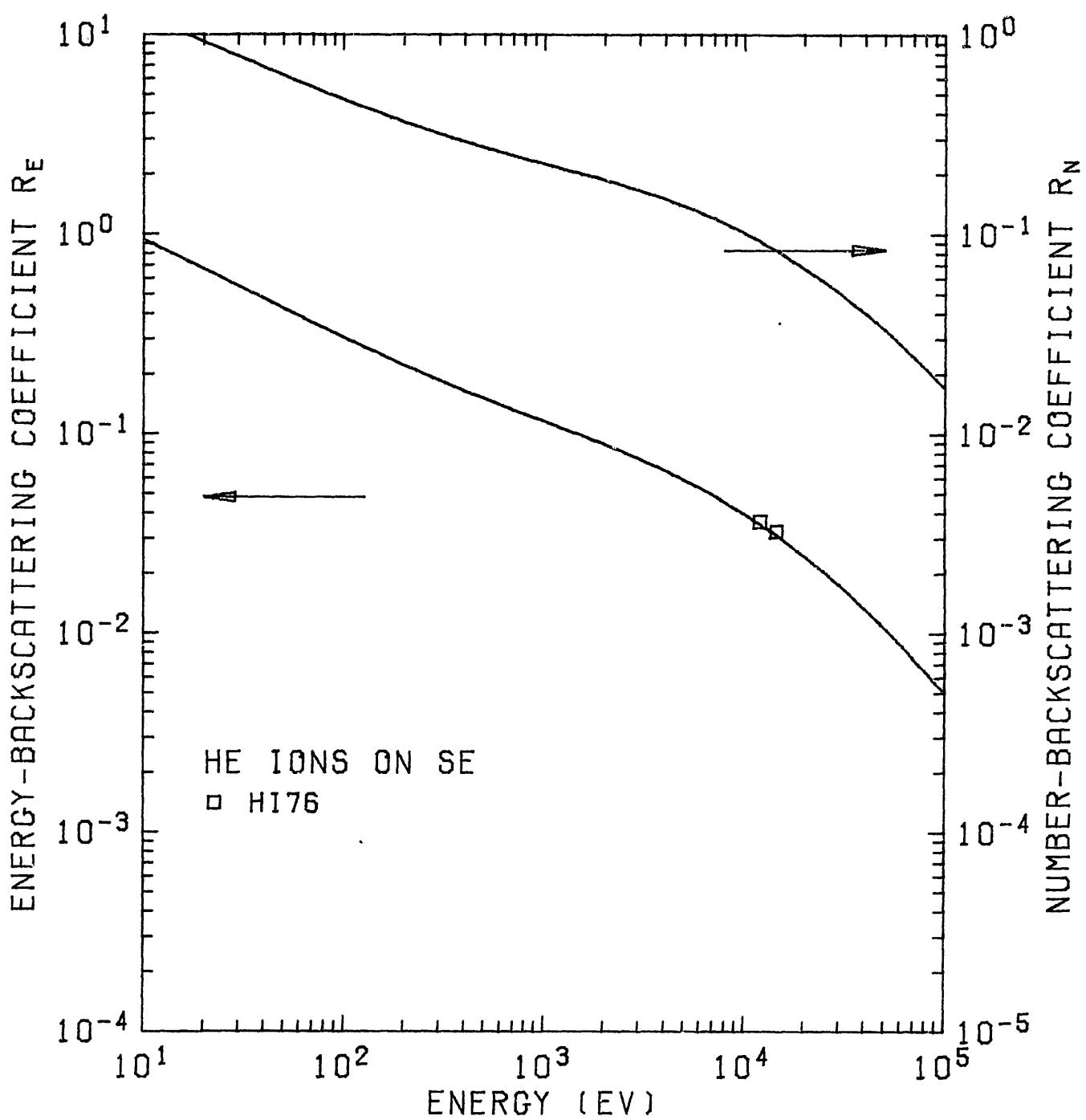
Fig. 39.  $R_N$  and  $R_E$  of He ions on  $^{34}\text{Se}$ .
