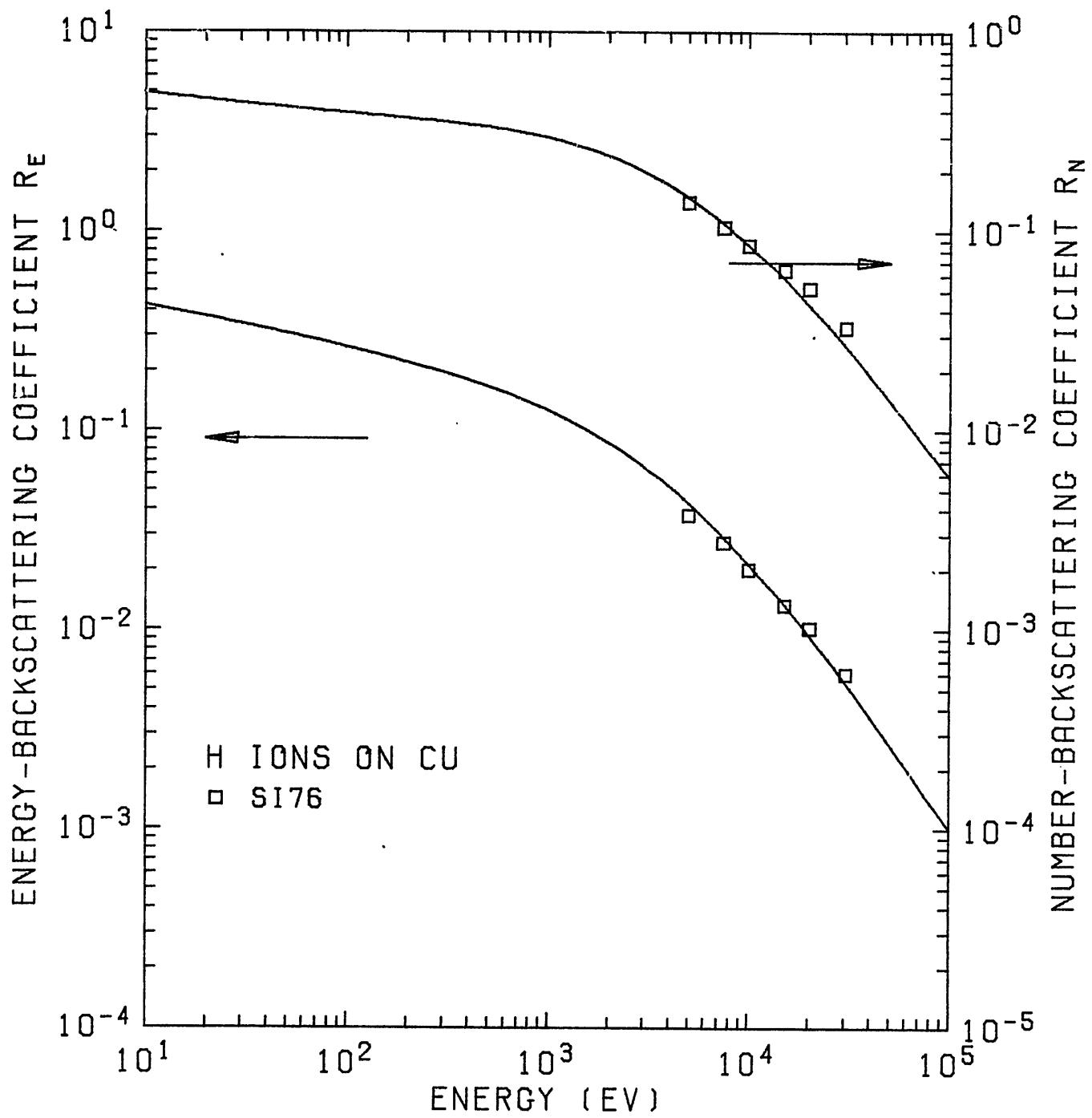
Fig. 7.  $R_N$  and  $R_E$  of H ions on  $^{29}\text{Cu}$ .
