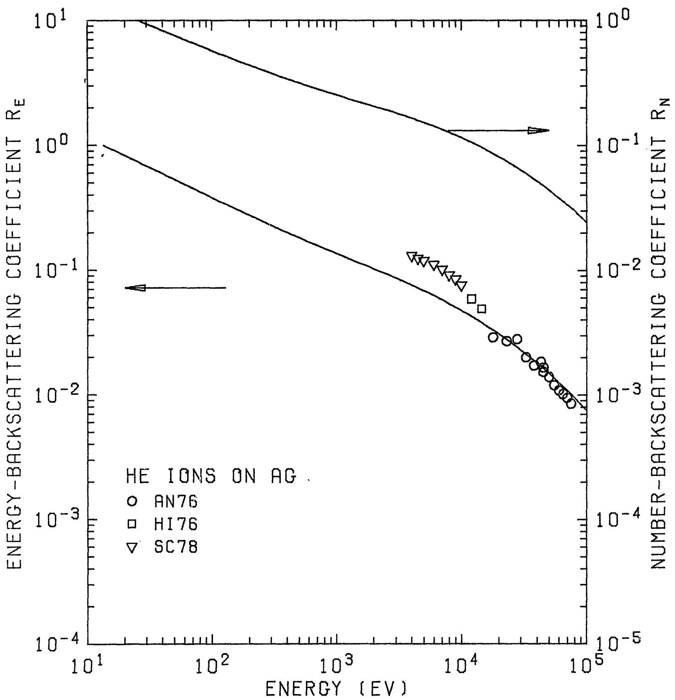
Fig. 44.  $R_N$  and  $R_E$  of He ions on  $^{47}\text{Ag}$ .
