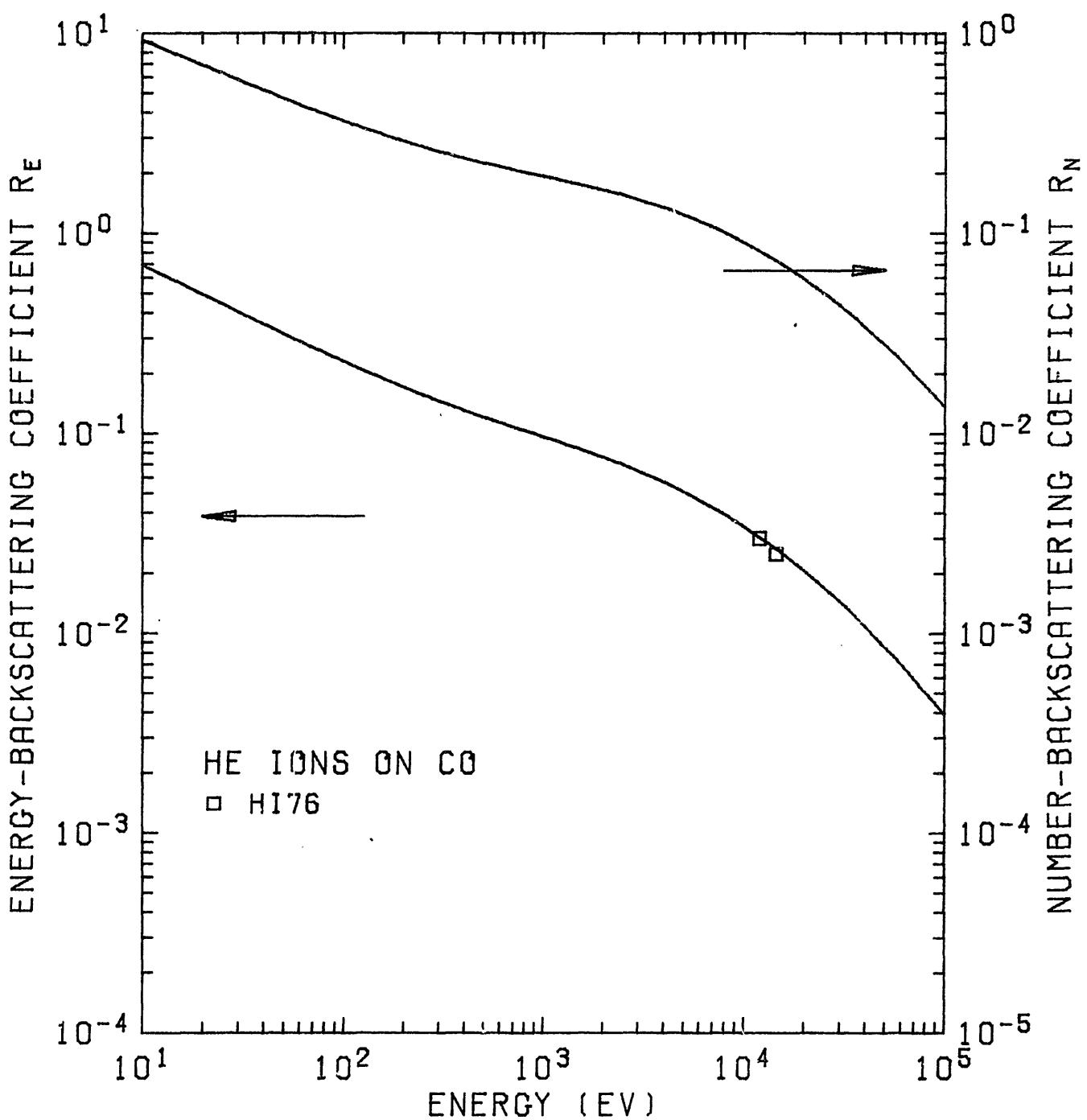
Fig. 33.  $R_N$  and  $R_E$  of He ions on  $^{27}\text{Co}$ .
