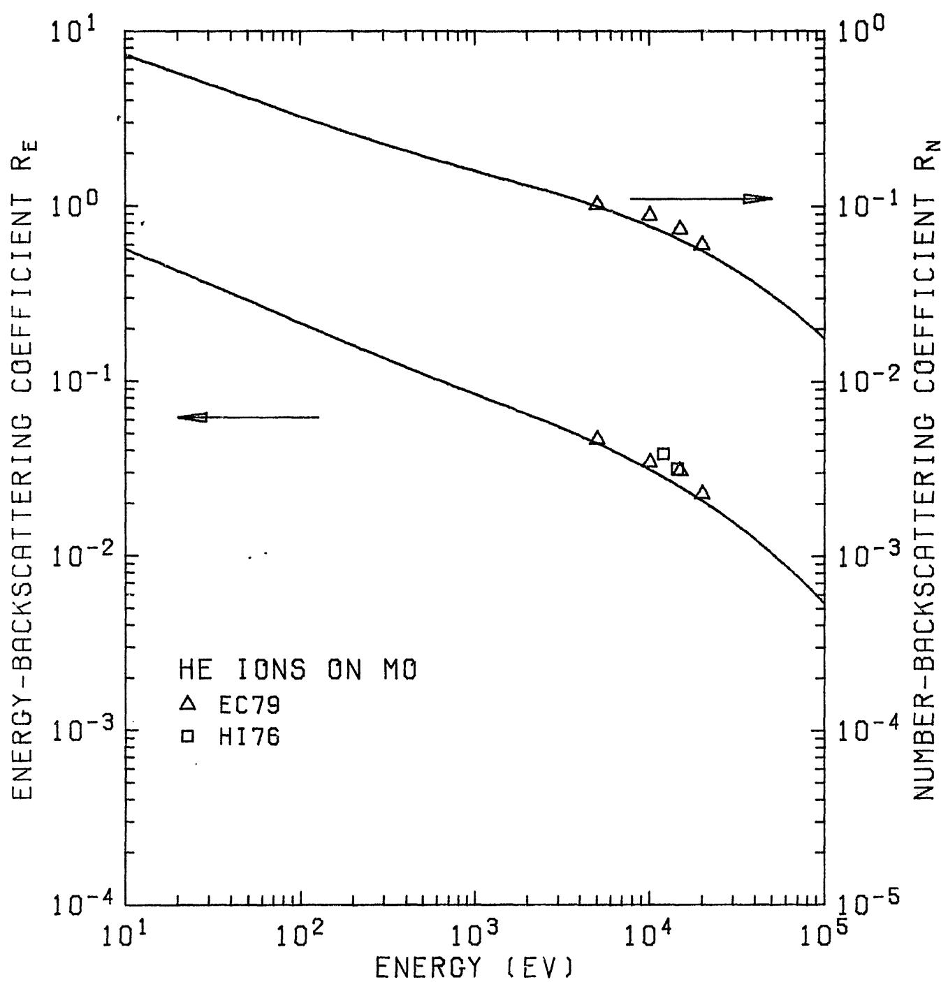
Fig. 42.  $R_N$  and  $R_E$  of He ions on  $^{42}\text{Mo}$ .
