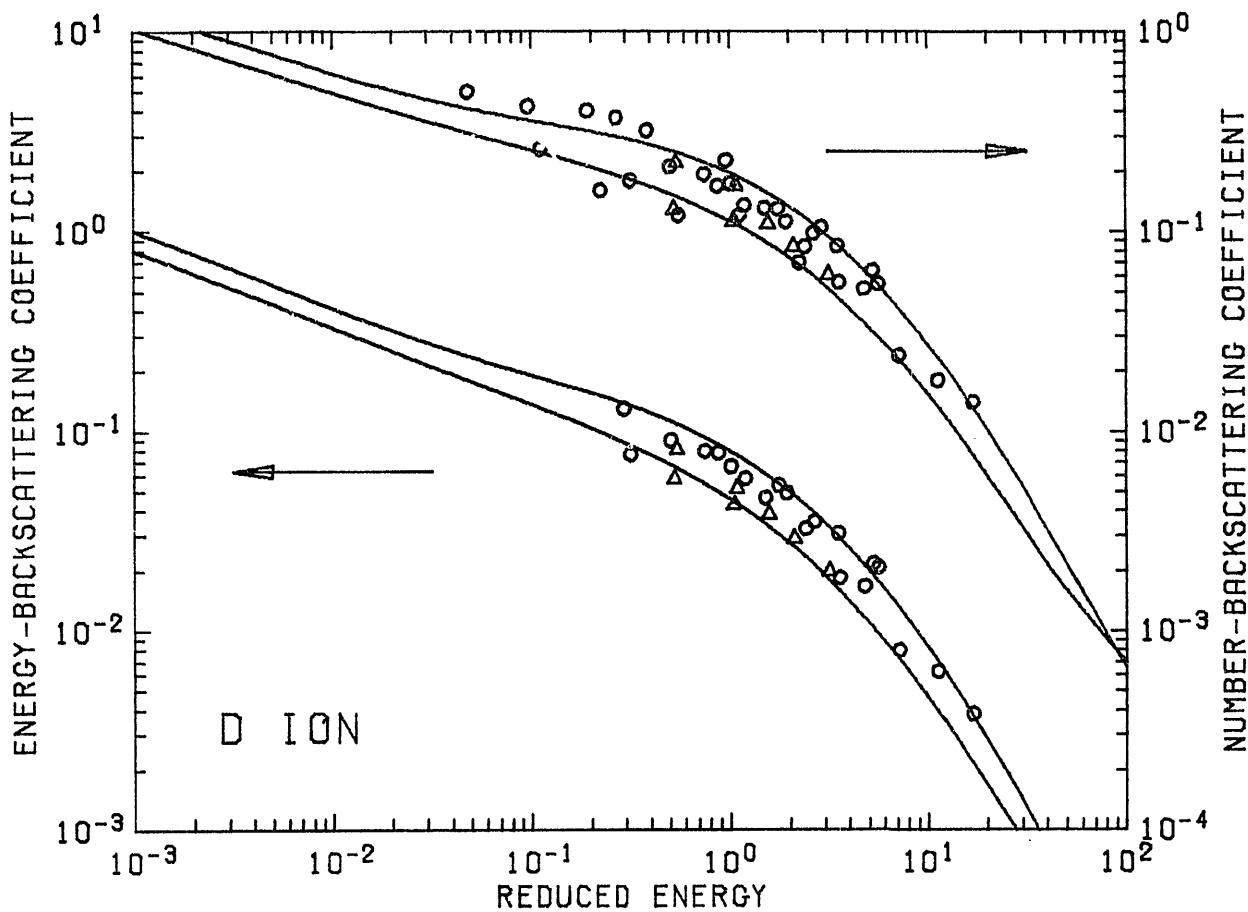
Fig. III.2. The number-backscattering coefficient  $R_N$  and the energy-backscattering coefficient  $R_E$  of D ions are plotted as a function of the Thomas-Fermi reduced energy  $\epsilon$ . o: experimental results for the targets of C, Ti, stainless steel, Ni, W, and Au; Δ: experimental results for the targets of Nb and Mo; curves: the empirical formulas for the targets of Fe (the upper of each pair) and Nb (the lower).
