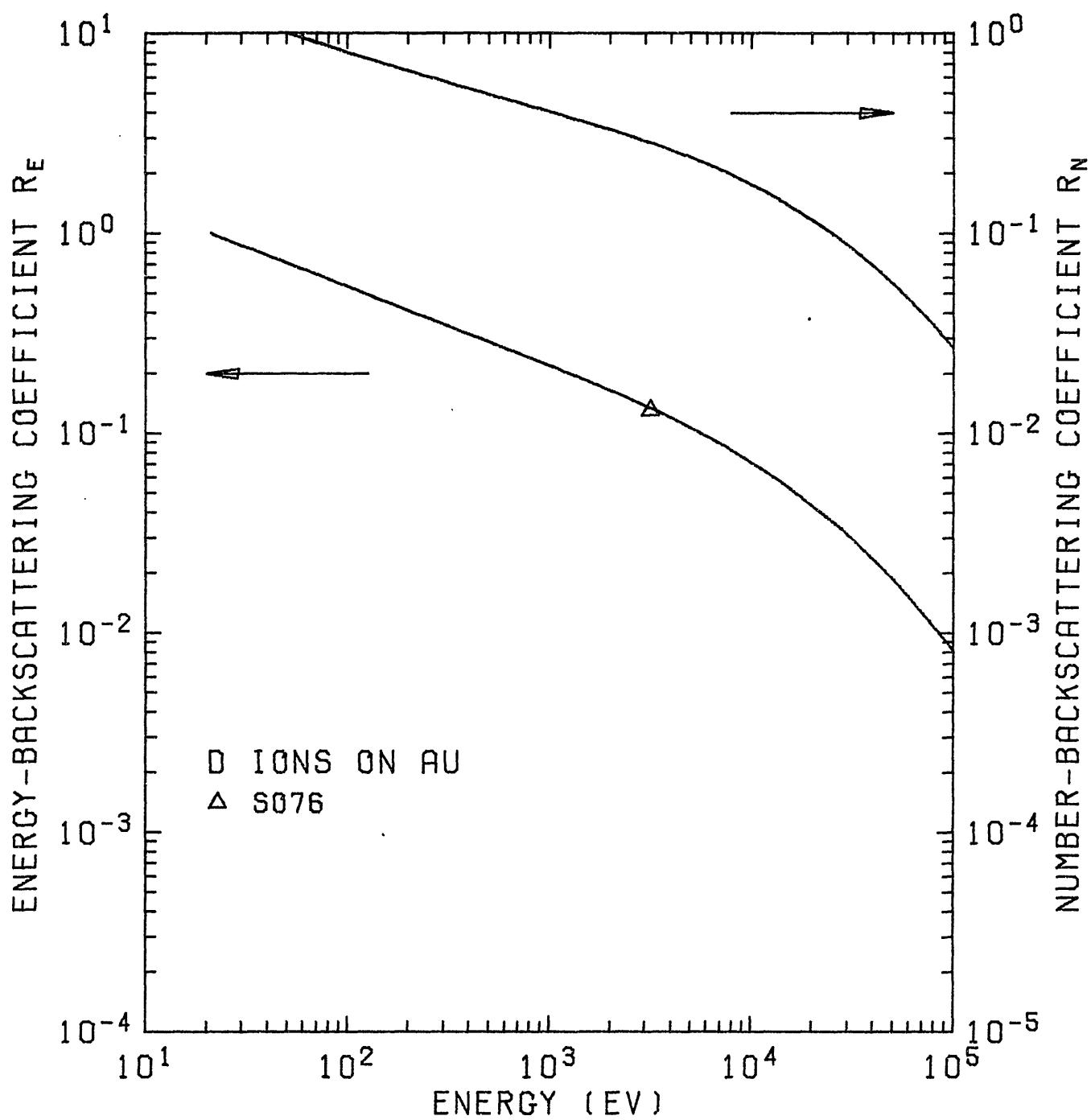
Fig. 23.  $R_N$  and  $R_E$  of D ions on  $^{79}\text{Au}$ .
