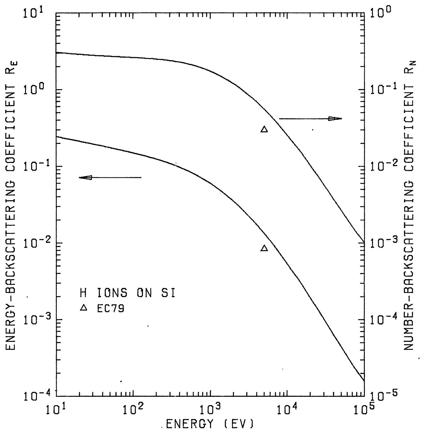
Fig. 3.  $R_N$  and  $R_E$  of H ions on  $^{14}\text{Si}$ .
