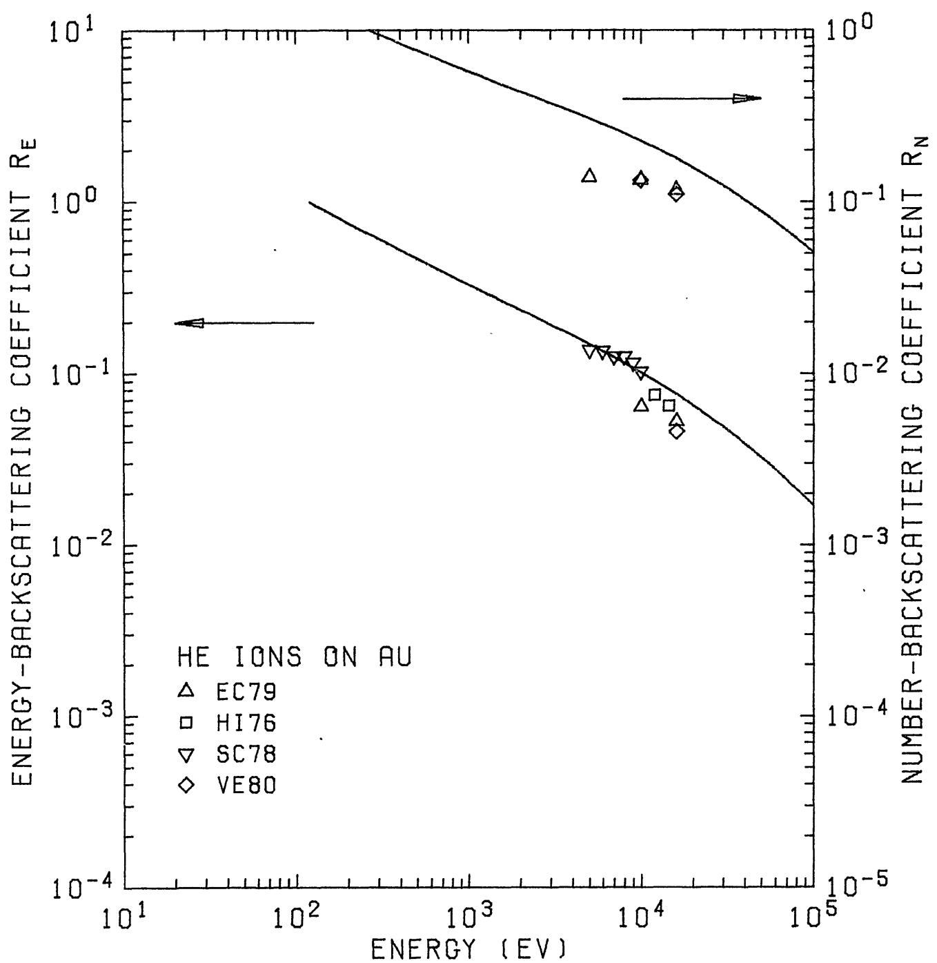
Fig. 53.  $R_N$  and  $R_E$  of He ions on  $^{79}\text{Au}$ .
