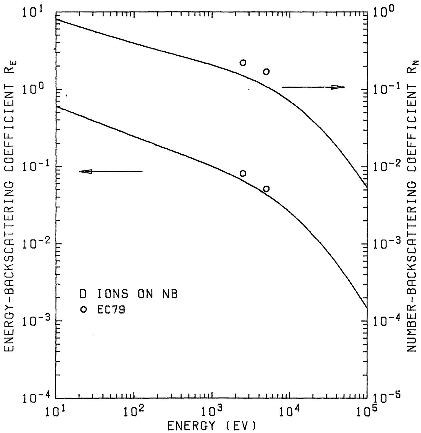
Fig. 20.  $R_N$  and  $R_E$  of D ions on  $_{41}\text{Nb}$ .
