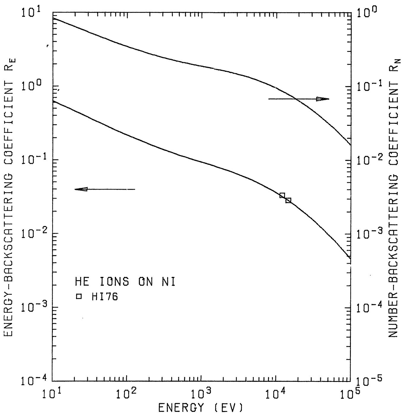
Fig. 34.  $R_N$  and  $R_E$  of He ions on  $^{28}\text{Ni}$ .
