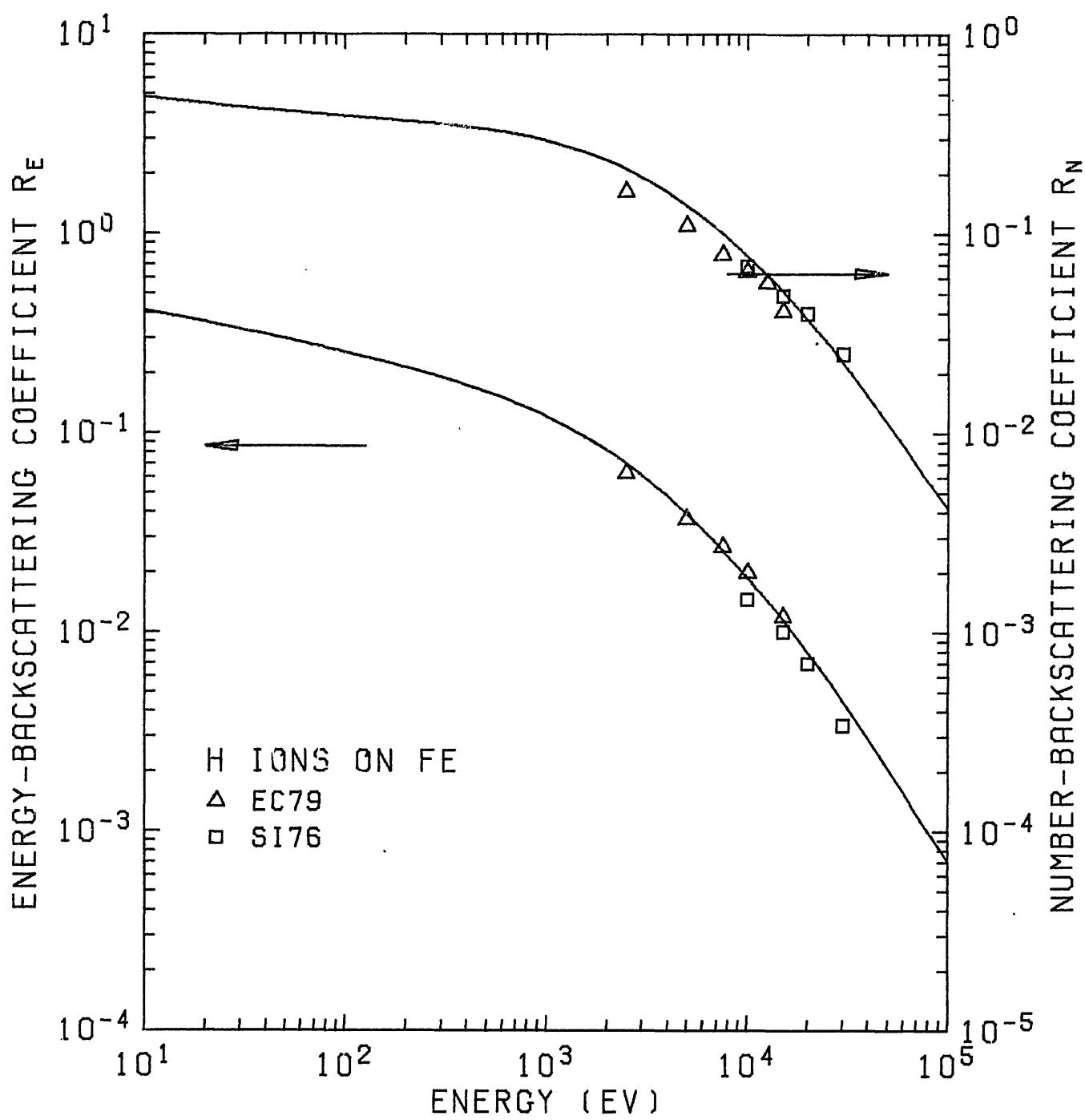
Fig. 5.  $R_N$  and  $R_E$  of H ions on  $^{26}\text{Fe}$ .
