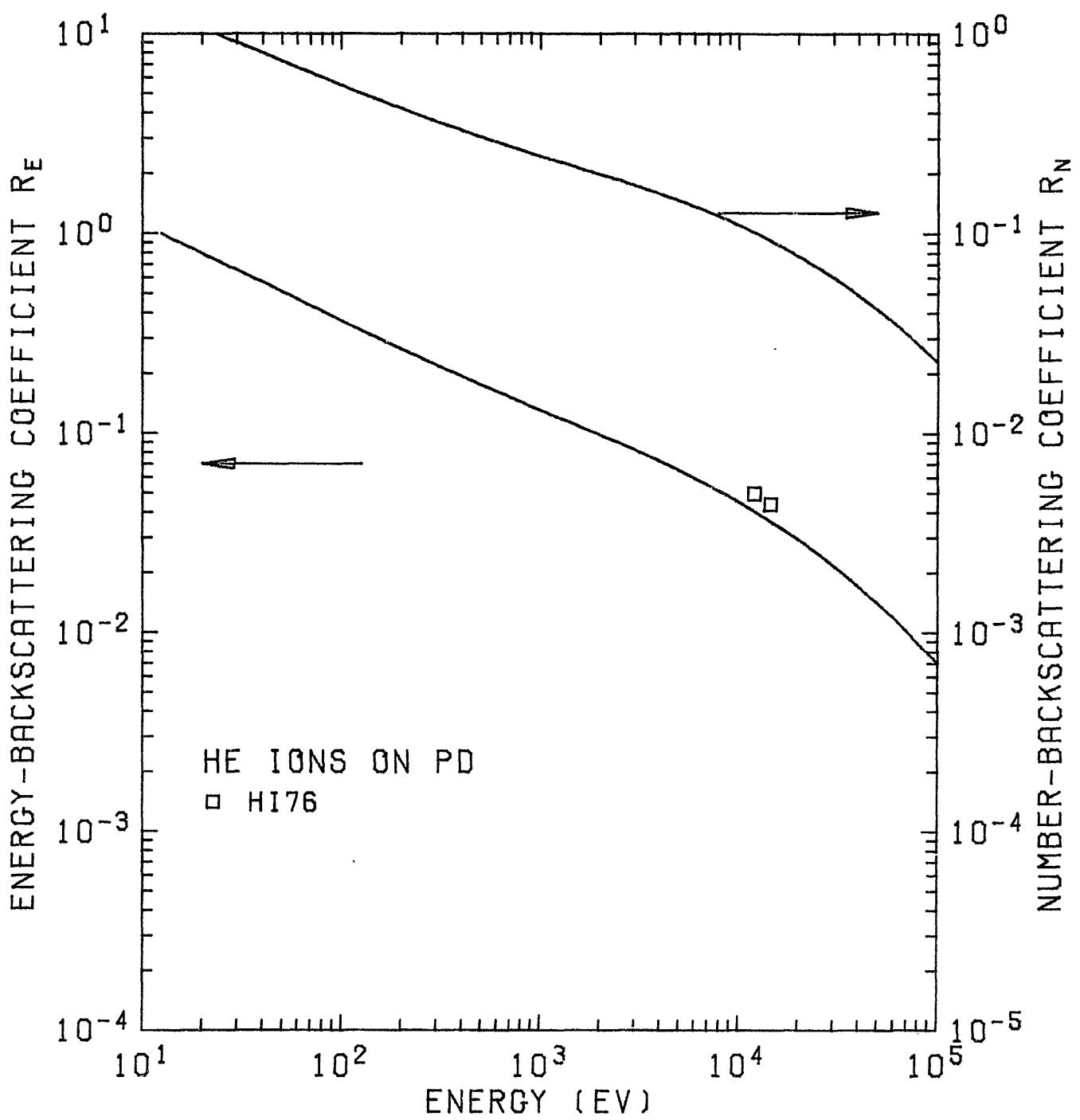
Fig. 43.  $R_N$  and  $R_E$  of He ions on  $^{46}\text{Pd}$ .
