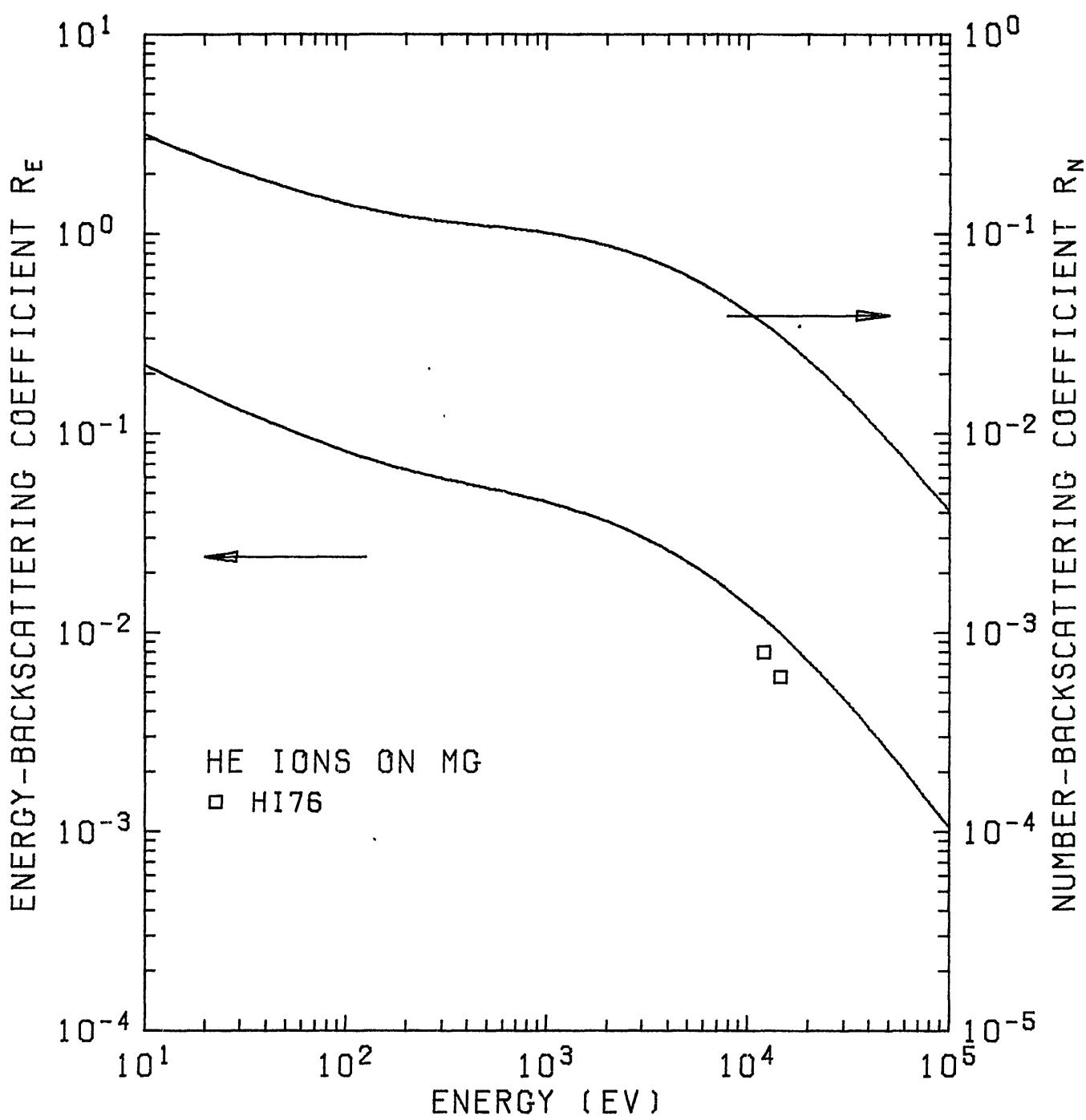
Fig. 25.  $R_N$  and  $R_E$  of He ions on  $^{12}\text{Mg}$ .
