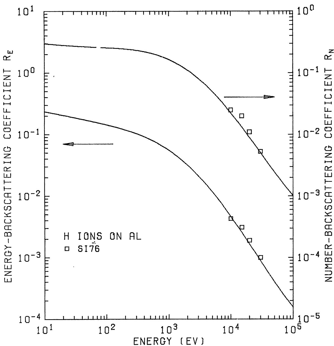
Fig. 2.  $R_N$  and  $R_E$  of H ions on  $^{13}\text{Al}$ .
