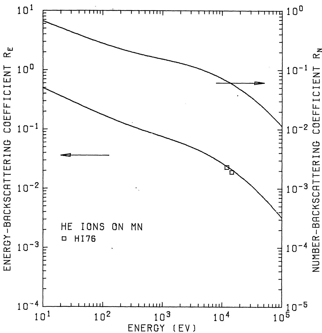
Fig. 31.  $R_N$  and  $R_E$  of He ions on  $^{25}\text{Mn}$ .
