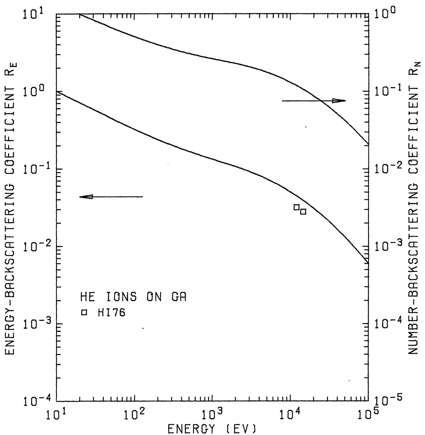
Fig. 37.  $R_N$  and  $R_E$  of He ions on  $_{31}\text{Ga}$ .
