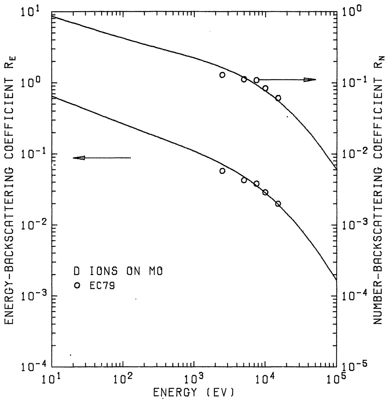
Fig. 21.  $R_N$  and  $R_E$  of D ions on  $^{42}\text{Mo}$ .
