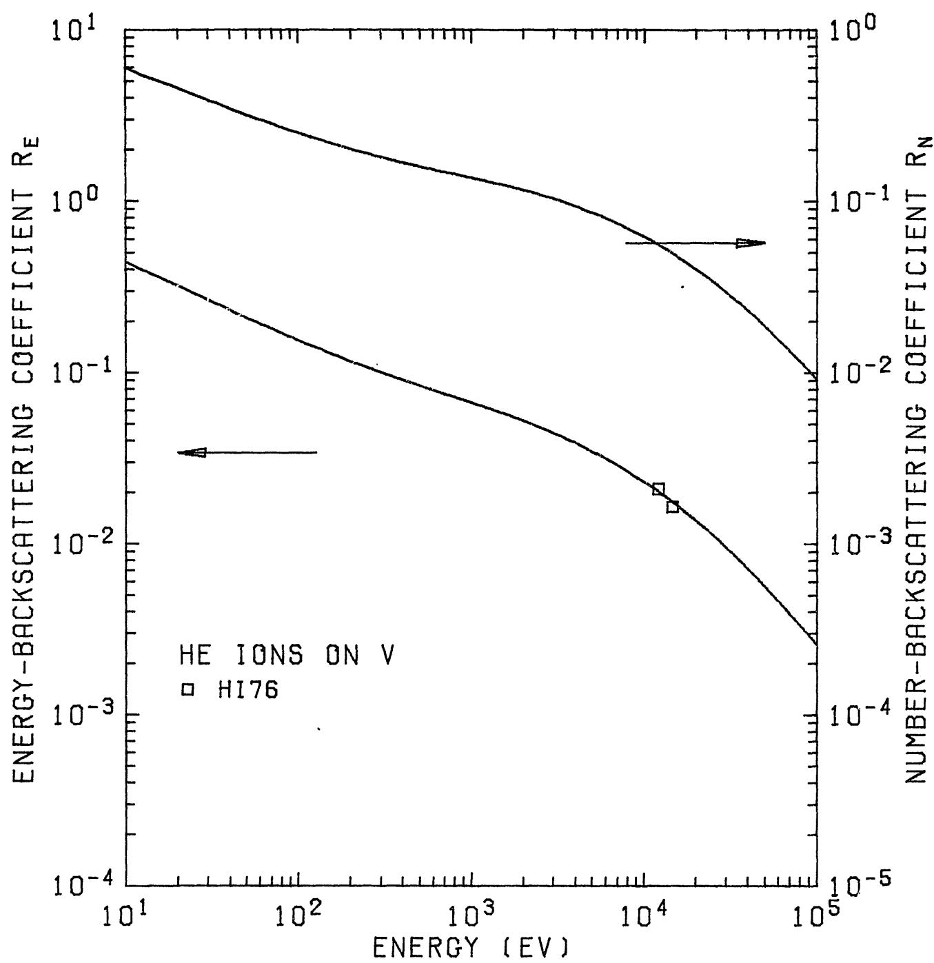
Fig. 29.  $R_N$  and  $R_E$  of He ions on  $^{23}V$ .
