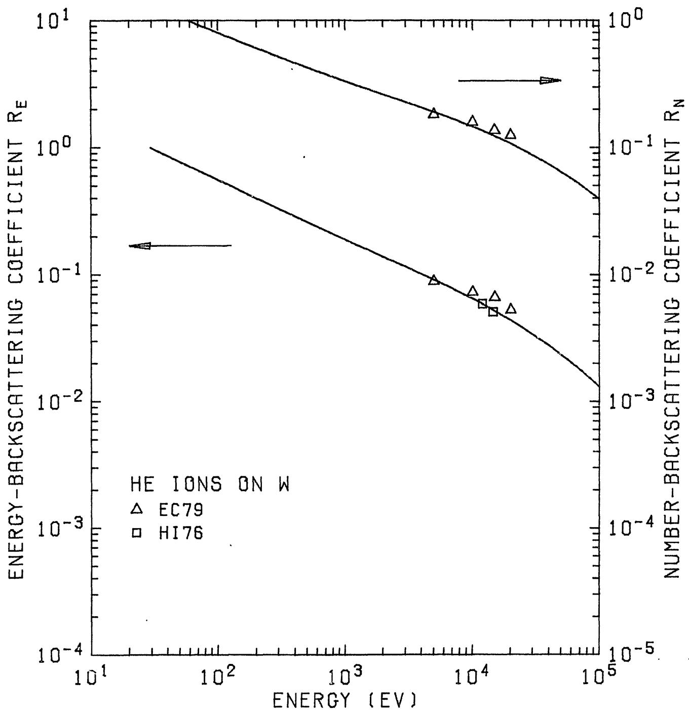
Fig. 51.  $R_N$  and  $R_E$  of He ions on  $^{74}W$ .
