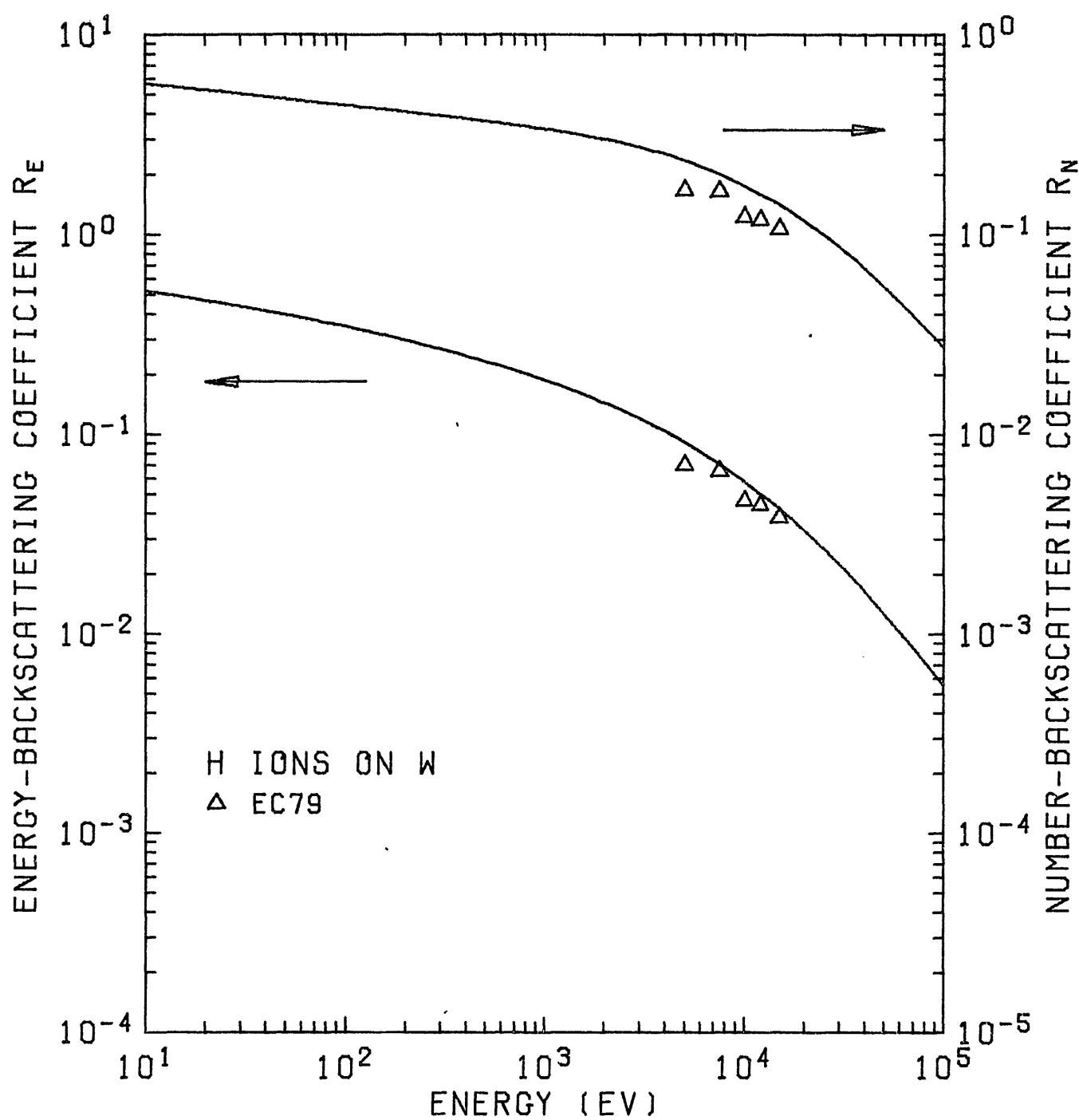
Fig. 13.  $R_N$  and  $R_E$  of H ions on  $^{74}W$ .
