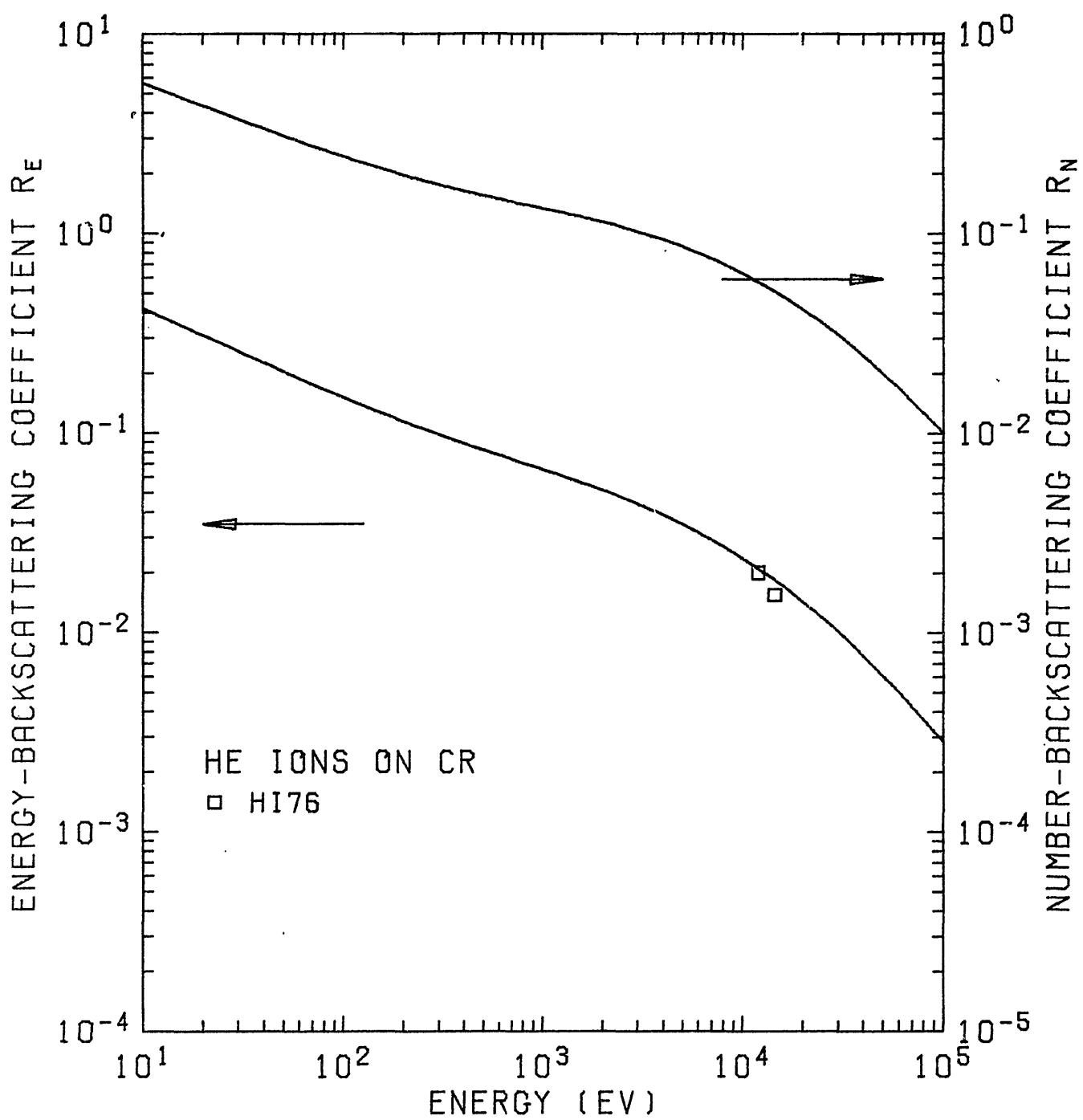
Fig. 30.  $R_N$  and  $R_E$  of He ions on  $^{24}\text{Cr}$ .
