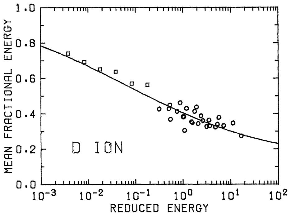
Fig. II.5. The mean fractional energy  $r_E$  of backscattered particles when D ions are incident is plotted as a function of the Thomas-Fermi reduced energy  $\epsilon$ . o: experimental results; squares: Monte Carlo results (ref. 3); curve: the empirical formula. This figure includes additional experimental data other than those shown in Fig. 6 of ref. 4.
