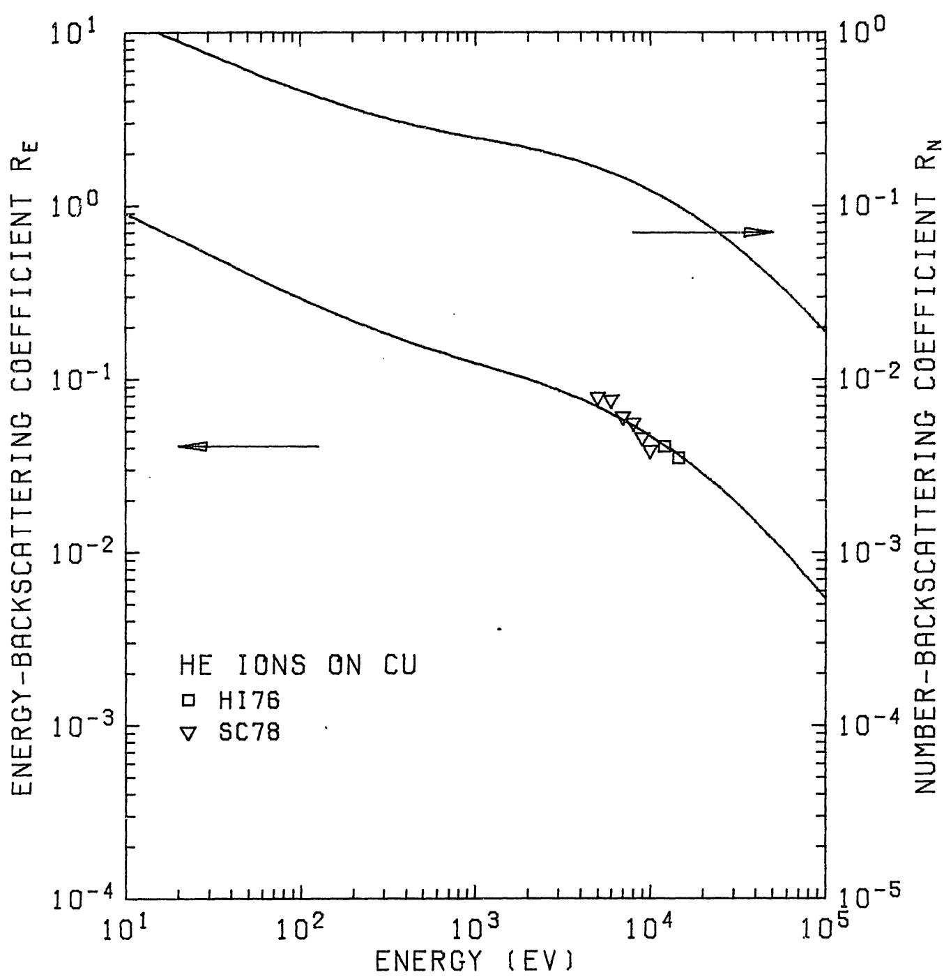
Fig. 35.  $R_N$  and  $R_E$  of He ions on  $^{29}\text{Cu}$ .
