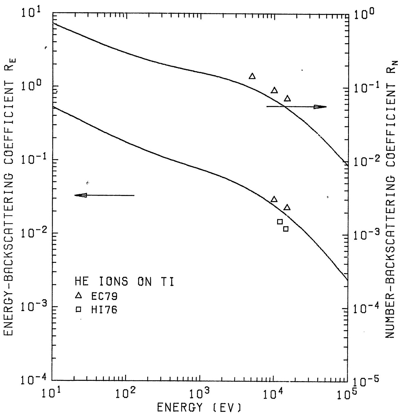
Fig. 28.  $R_N$  and  $R_E$  of He ions on  $^{22}\text{Ti}$ .
