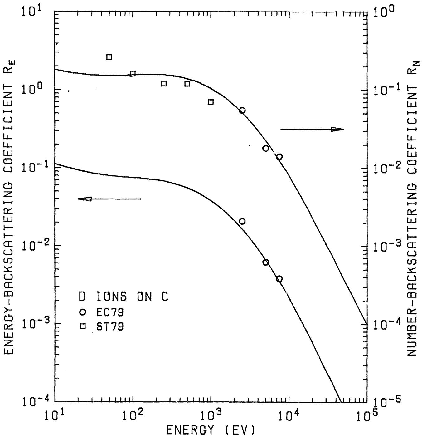
Fig. 16.  $R_N$  and  $R_E$  of D ions on  $^{12}\text{C}$ .
