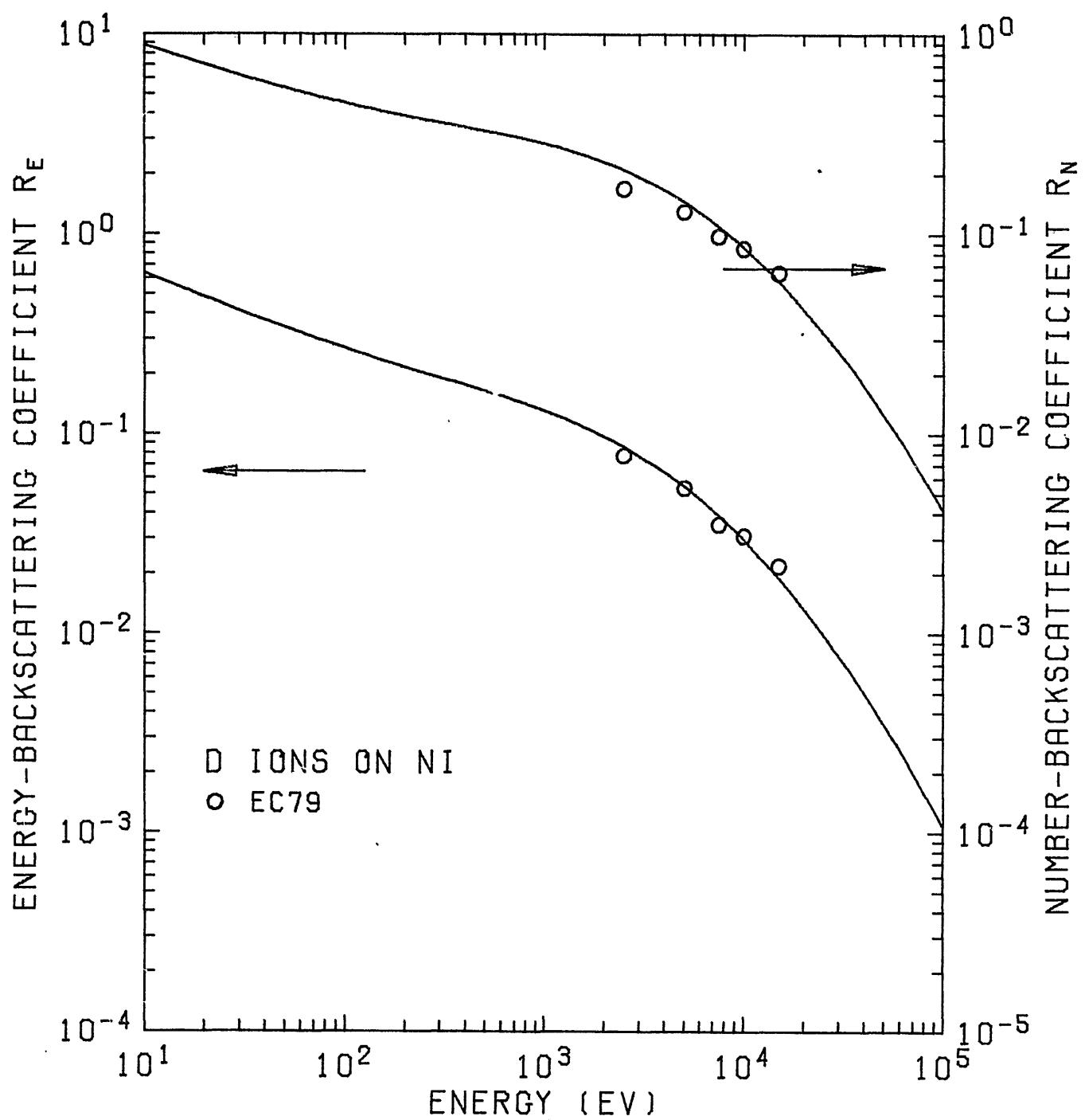
Fig. 19.  $R_N$  and  $R_E$  of D ions on  $^{28}\text{Ni}$ .
