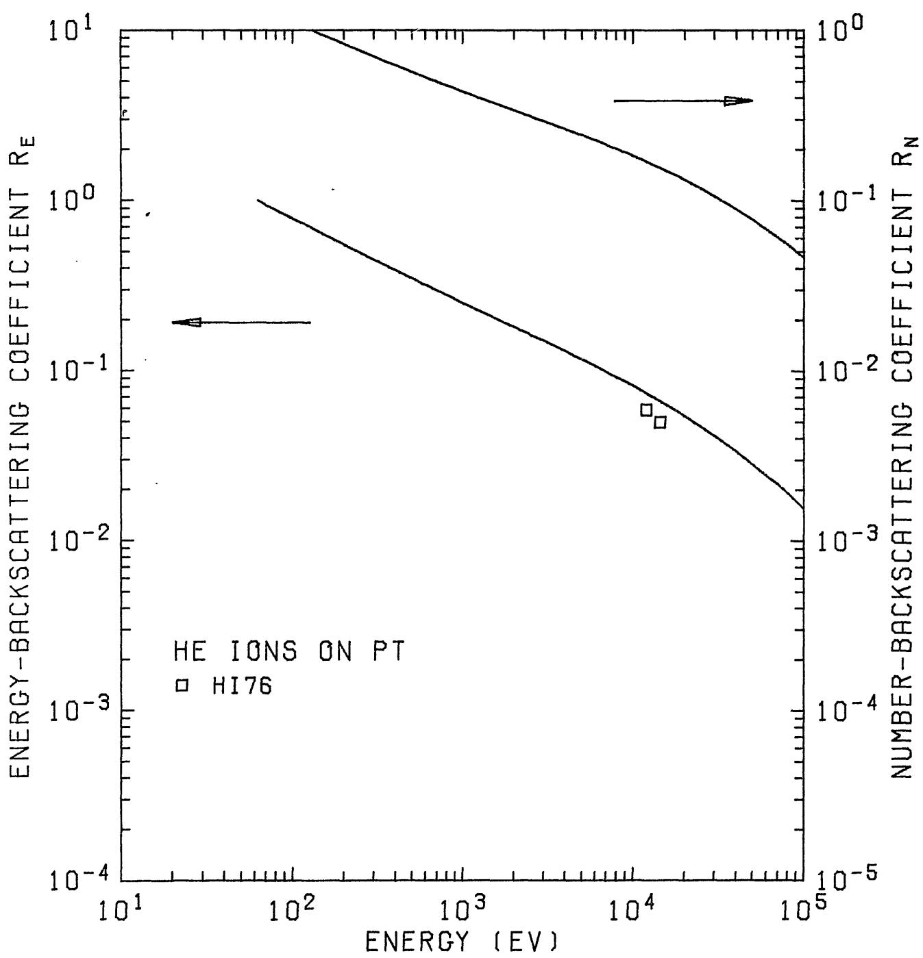
Fig. 52.  $R_N$  and  $R_E$  of He ions on  $^{78}\text{Pt}$ .
