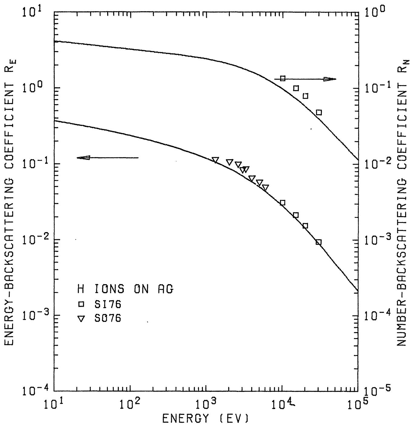
Fig. 11.  $R_N$  and  $R_E$  of H ions on  $^{47}\text{Ag}$ .
