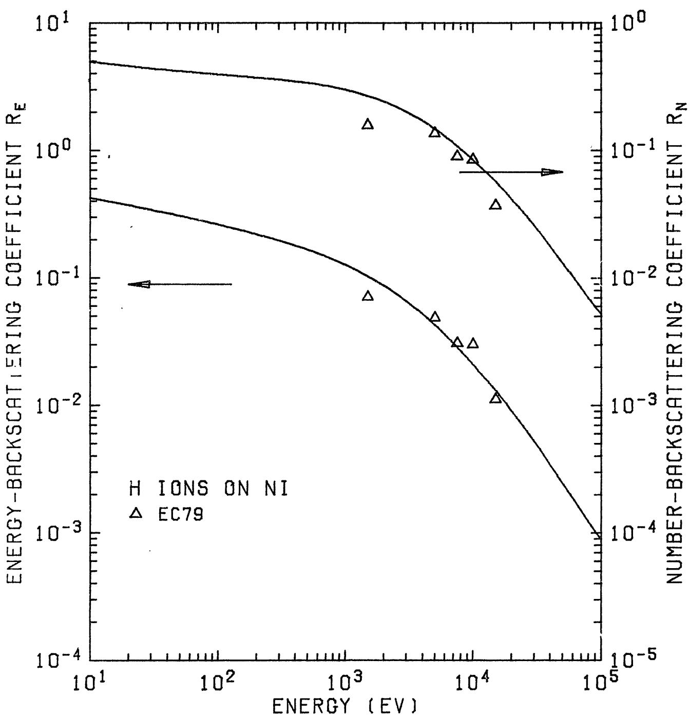
Fig. 6.  $R_N$  and  $R_E$  of H ions on  $^{28}\text{Ni}$ .
