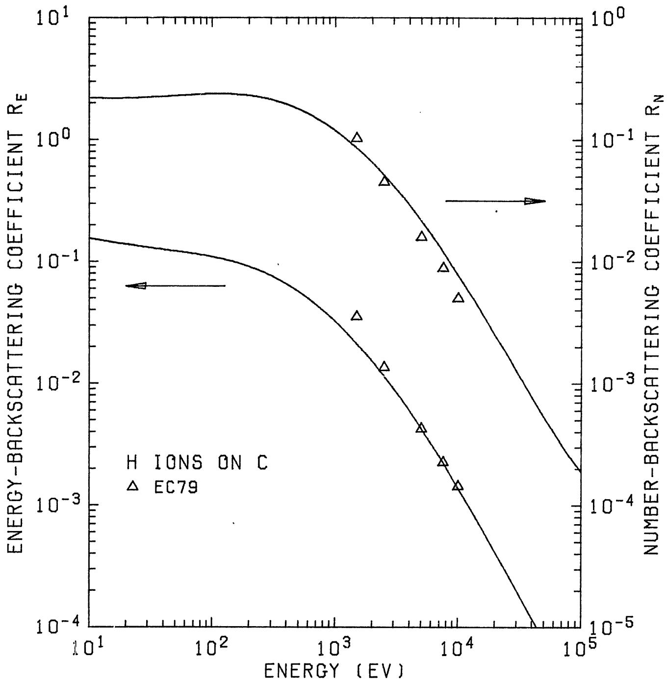
Fig. 1.  $R_N$  and  $R_E$  of H ions on  $^{64}\text{C}$ .
