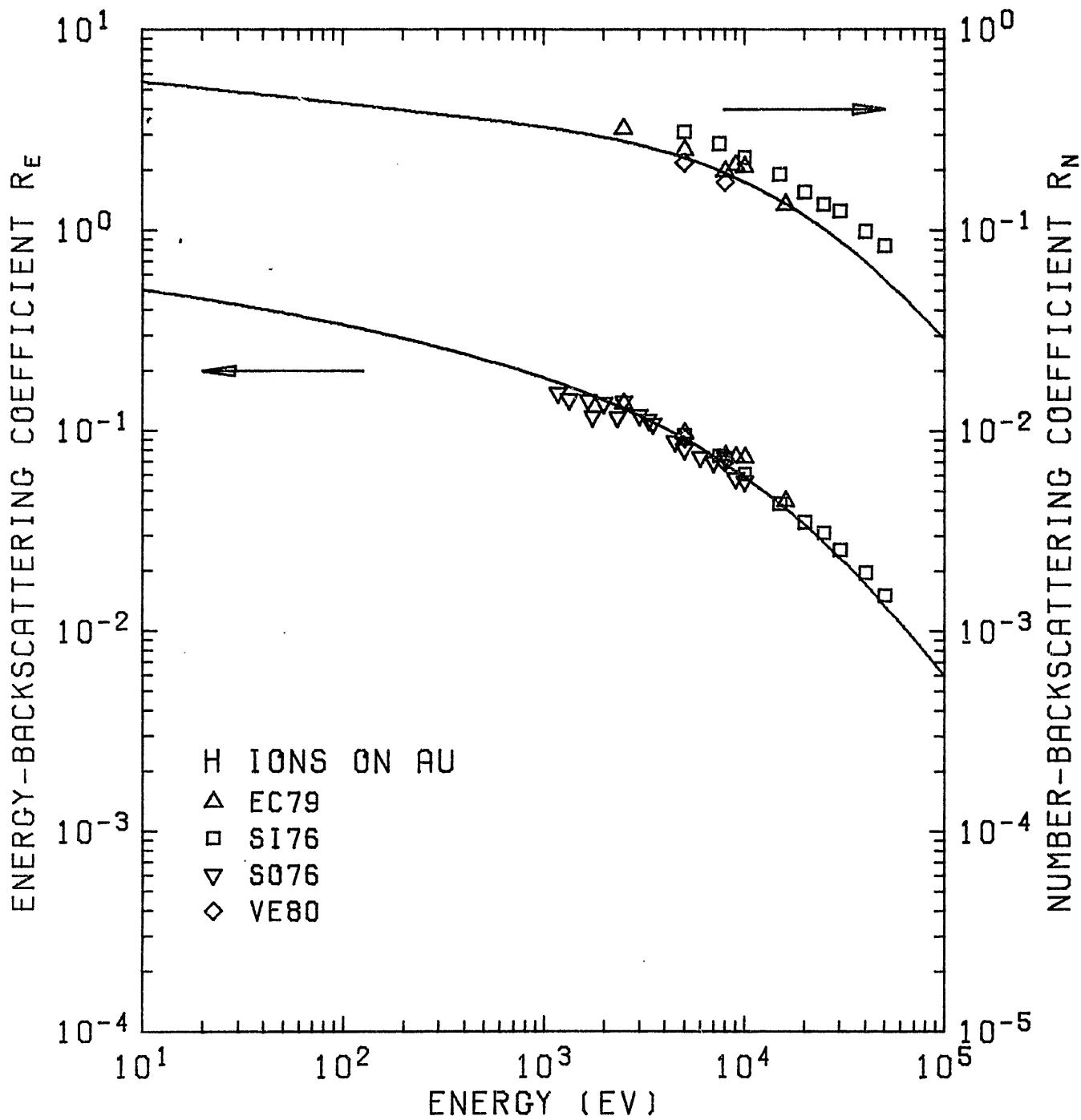
Fig. 14.  $R_N$  and  $R_E$  of H ions on  $^{79}\text{Au}$ .
