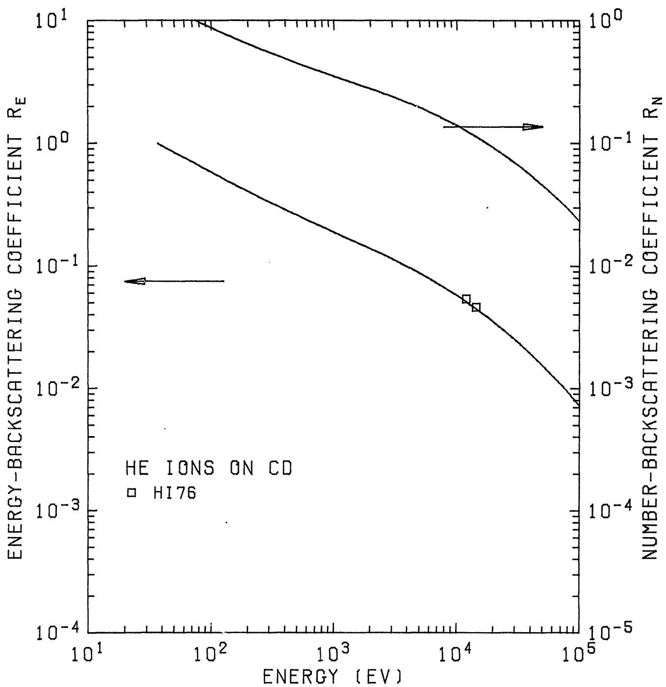
Fig. 45.  $R_N$  and  $R_E$  of He ions on  $^{48}\text{Cd}$ .
