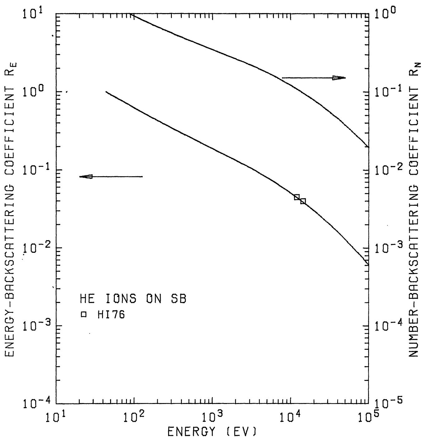
Fig. 48.  $R_N$  and  $R_E$  of He ions on  $^{51}\text{Sb}$ .
