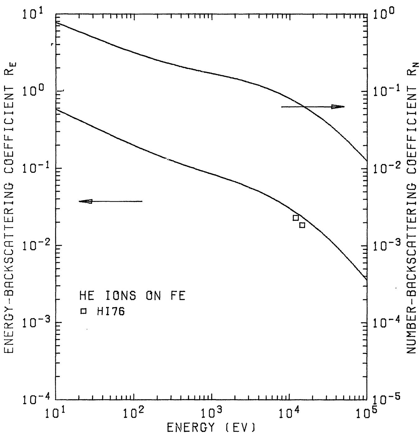
Fig. 32.  $R_N$  and  $R_E$  of He ions on  $^{26}\text{Fe}$ .
