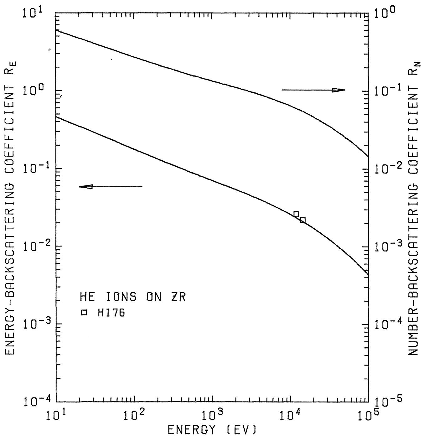
Fig. 40.  $R_N$  and  $R_E$  of He ions on  $_{40}\text{Zr}$ .
