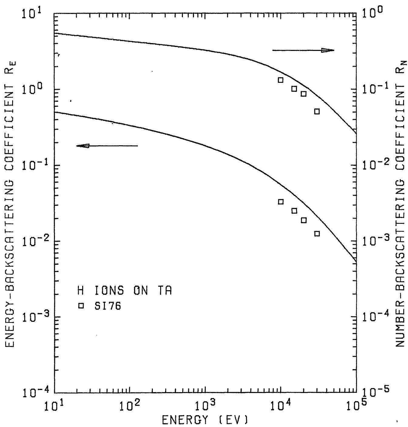
Fig. 12.  $R_N$  and  $R_E$  of  $H$  ions on  $_{73}Ta$ .
