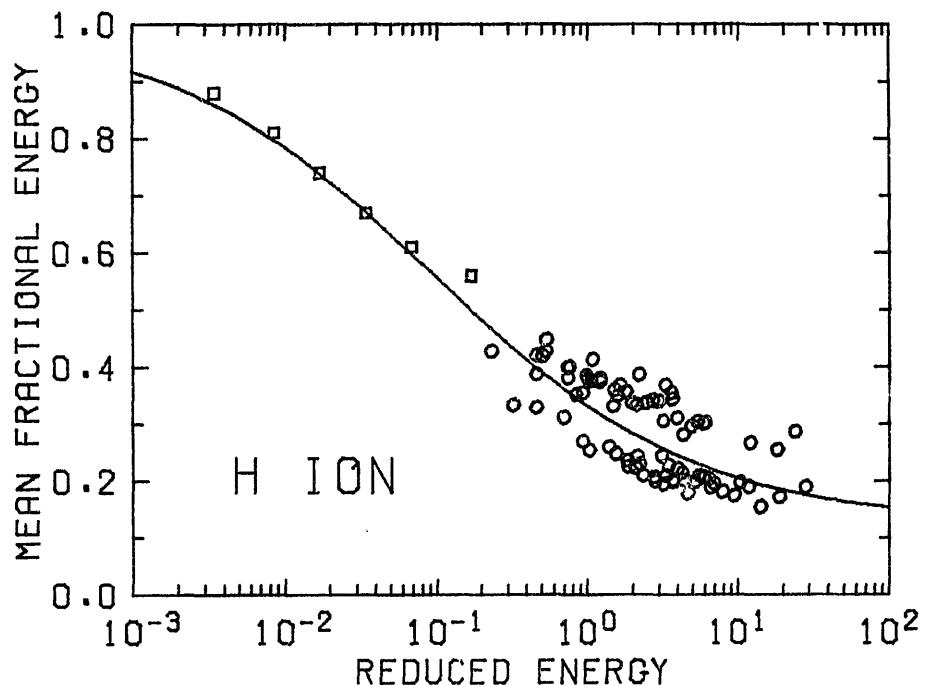
Fig. II.4. The mean fractional energy  $r_E$  of backscattered particles when H ions are incident is plotted as a function of the Thomas-Fermi reduced energy  $\varepsilon$ . o: experimental results; squares: Monte Carlo results (ref. 5); curve: the empirical formula. This figure includes additional experimental data other than those shown in Fig. 5 of ref. 4.
