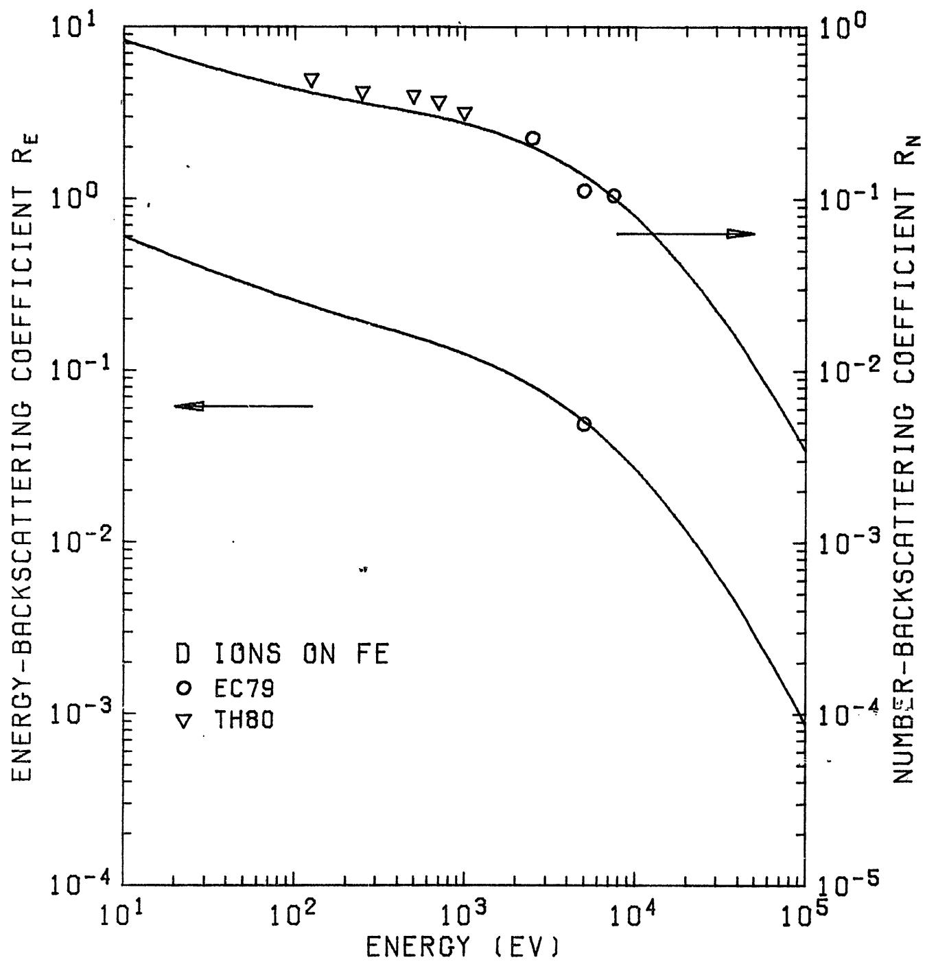
Fig. 18.  $R_N$  and  $R_E$  of D ions on  $^{26}\text{Fe}$ .
