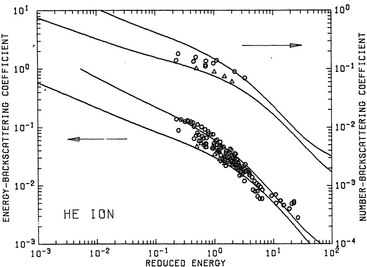
Fig. III.3. The number-backscattering coefficient  $R_N$  and the energy-backscattering coefficient  $R_E$  of He ions are plotted as a function of the Thomas-Fermi reduced energy  $\epsilon$ .  $\circ$ : experimental results for the targets of Si, Ti, Cu, Ag, W, Au, Pb and other twenty-one elemental materials;  $\Delta$ : experimental results for the targets of Nb, Mo and Ta; curves: the empirical formulas for the targets of Au (the upper of each pair) and Nb (the lower).
