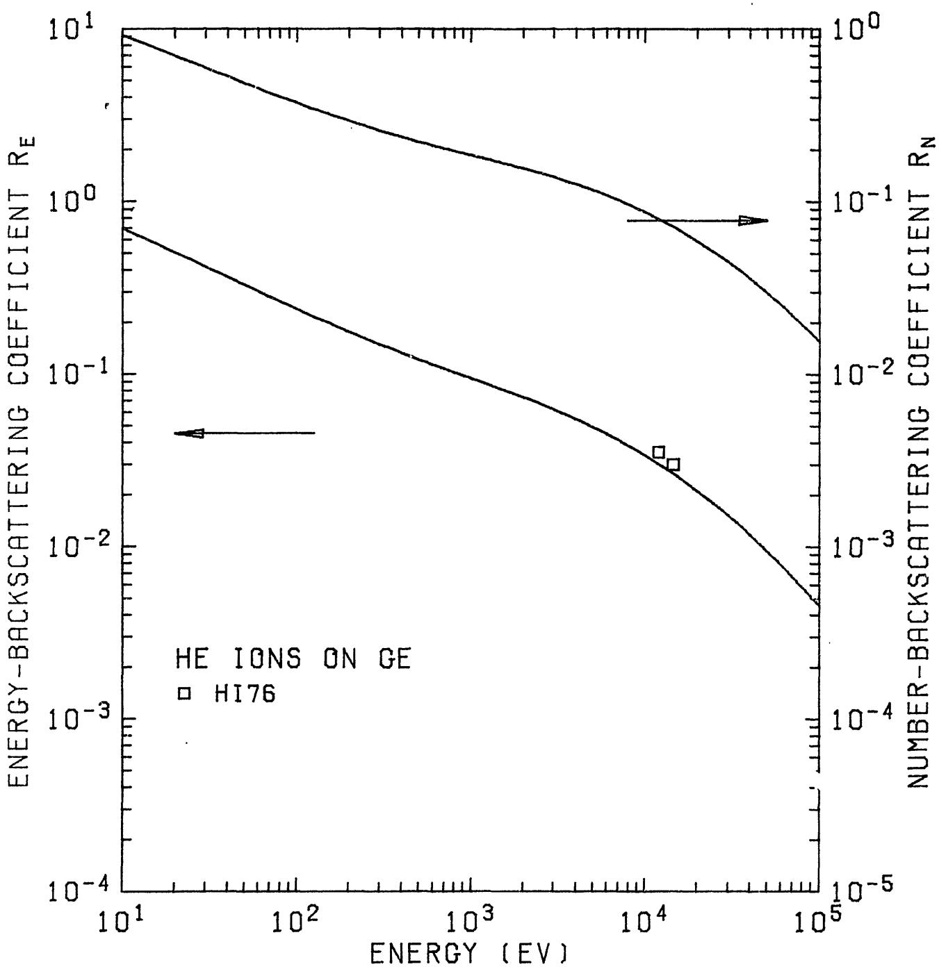
Fig. 38.  $R_N$  and  $R_E$  of He ions on  $^{32}\text{Ge}$ .
