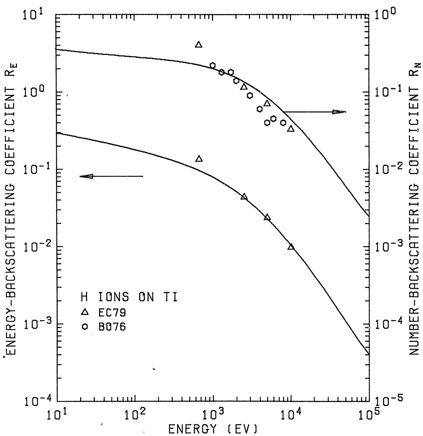
Fig. 4.  $R_N$  and  $R_E$  of H ions on  $^{22}\text{Ti}$ .
