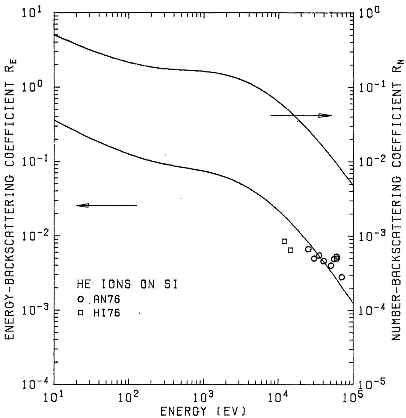
Fig. 27.  $R_N$  and  $R_E$  of He ions on  $^{14}\text{Si}$ .
