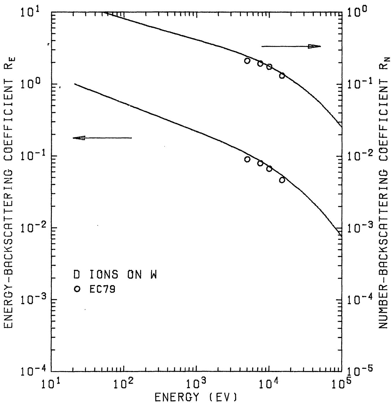
Fig. 22.  $R_N$  and  $R_E$  of D ions on  $_{74}W$ .
