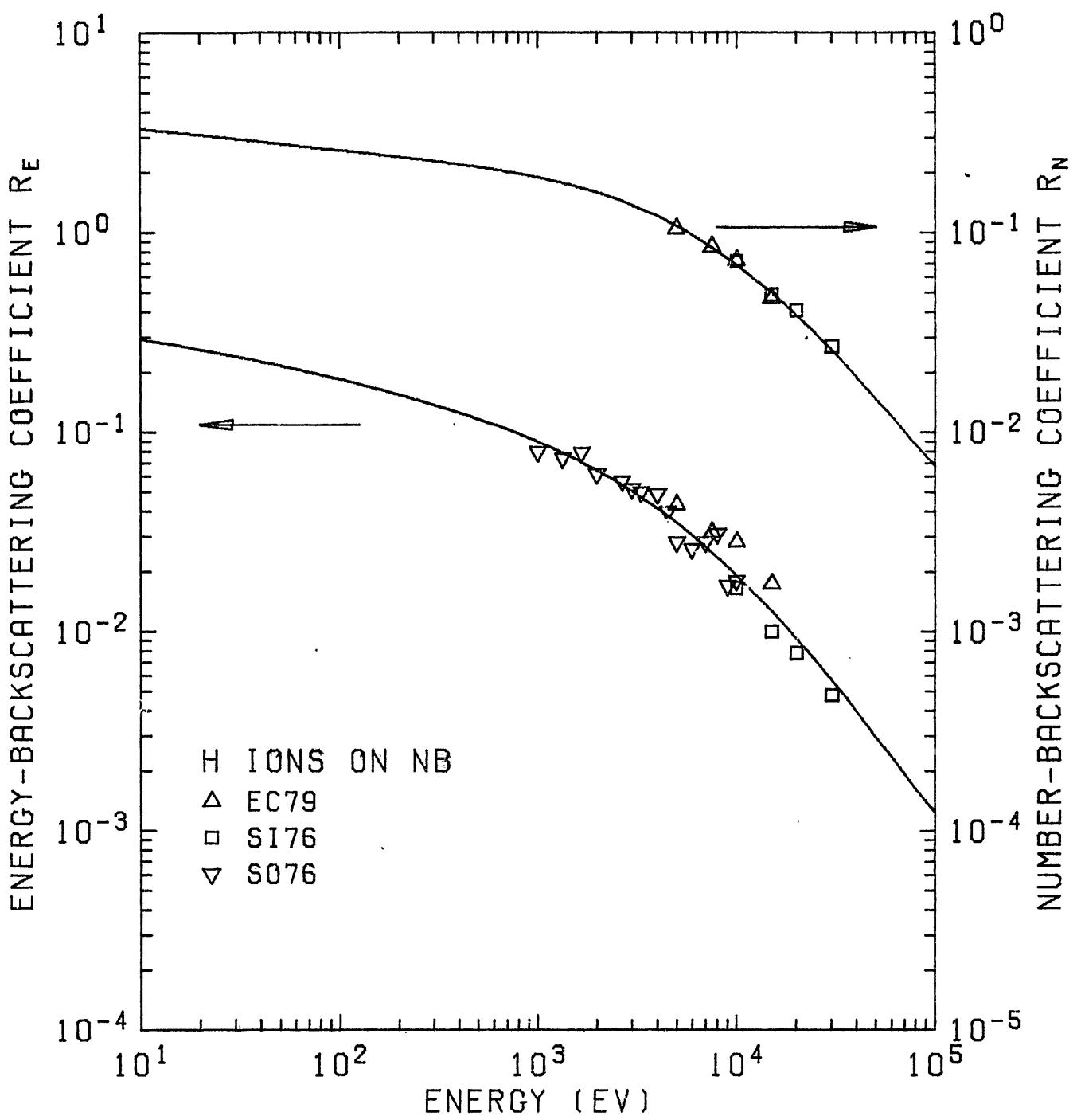
Fig. 9.  $R_N$  and  $R_E$  of H ions on  $_{41}\text{Nb}$ .
