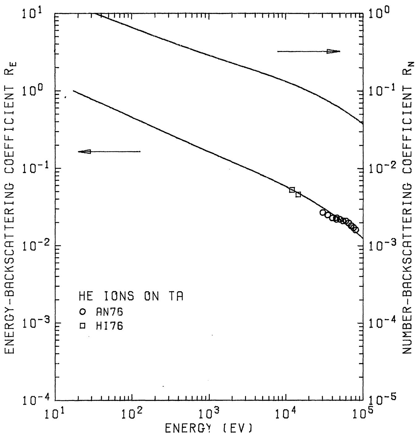
Fig. 50.  $R_N$  and  $R_E$  of He ions on  $_{73}\text{Ta}$ .
