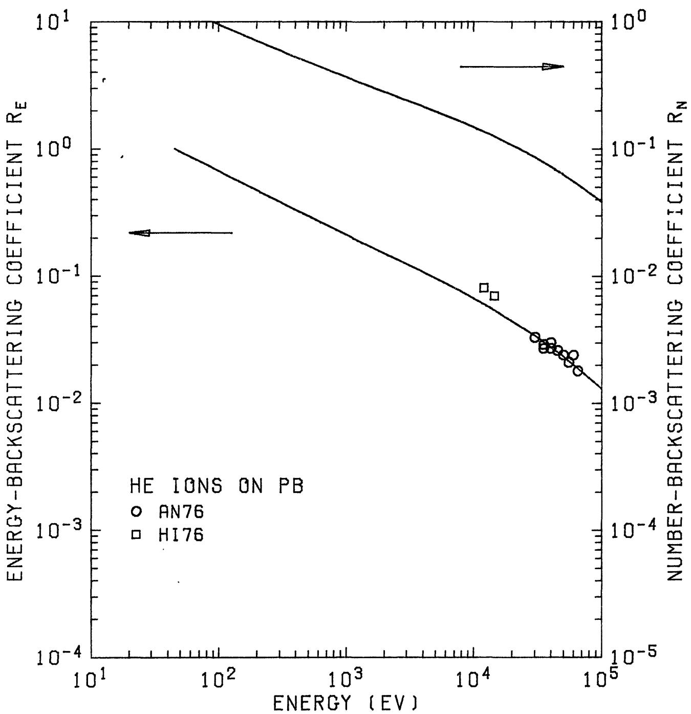
Fig. 54.  $R_N$  and  $R_E$  of He ions on  $^{82}\text{Pb}$ .
