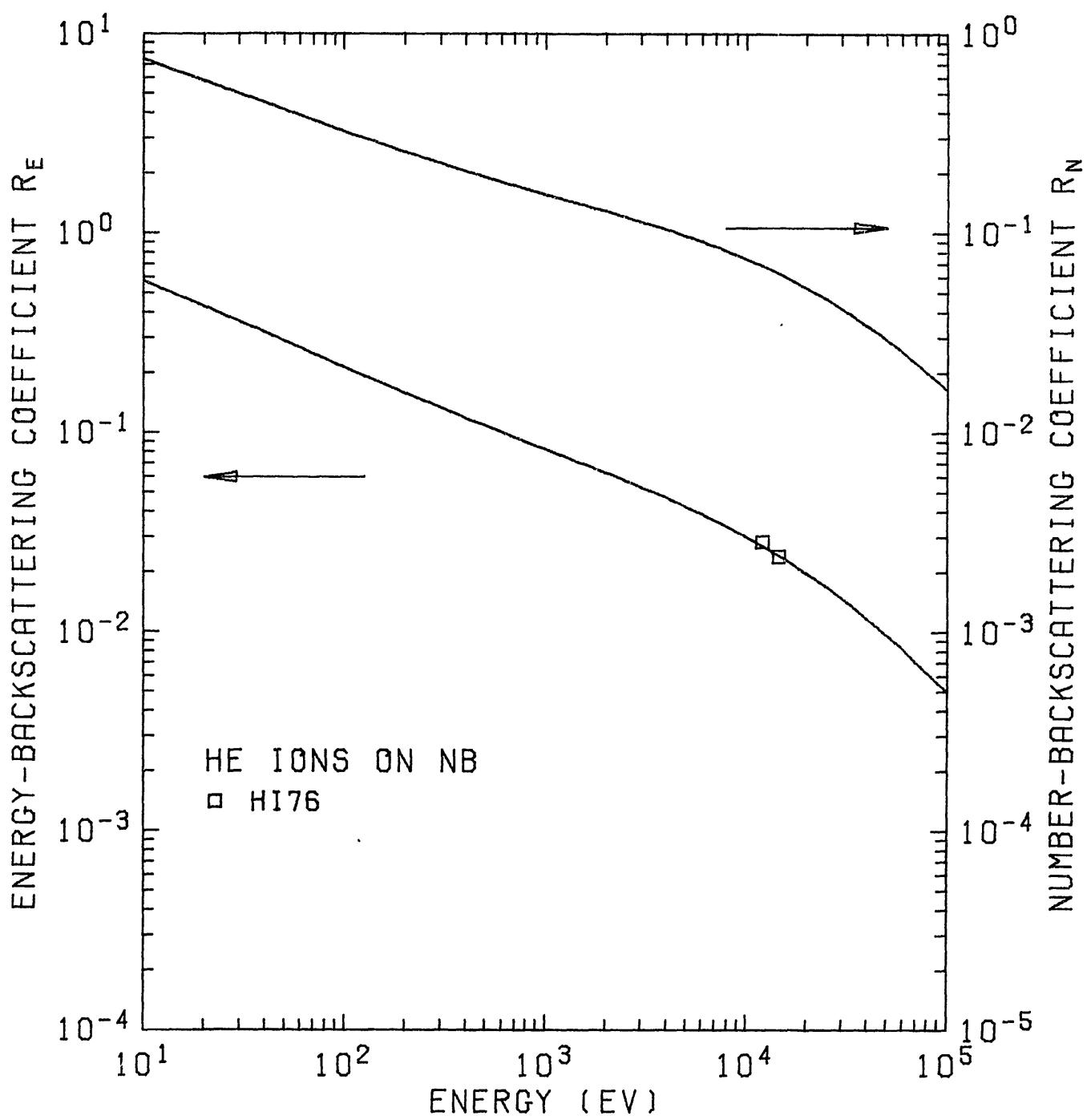
Fig. 41.  $R_N$  and  $R_E$  of He ions on  $_{41}\text{Nb}$ .
