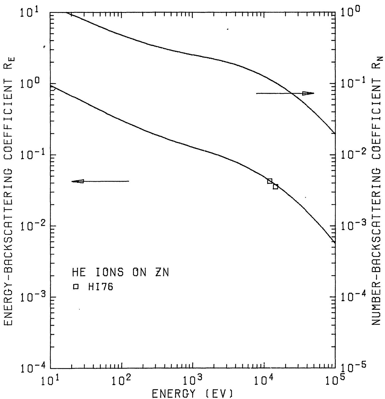
Fig. 36.  $R_N$  and  $R_E$  of He ions on  ${}_{30}\text{Zn}$ .
