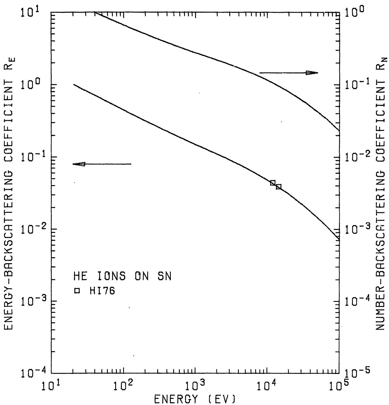
Fig. 47.  $R_N$  and  $R_E$  of He ions on  $^{50}\text{Sn}$ .
