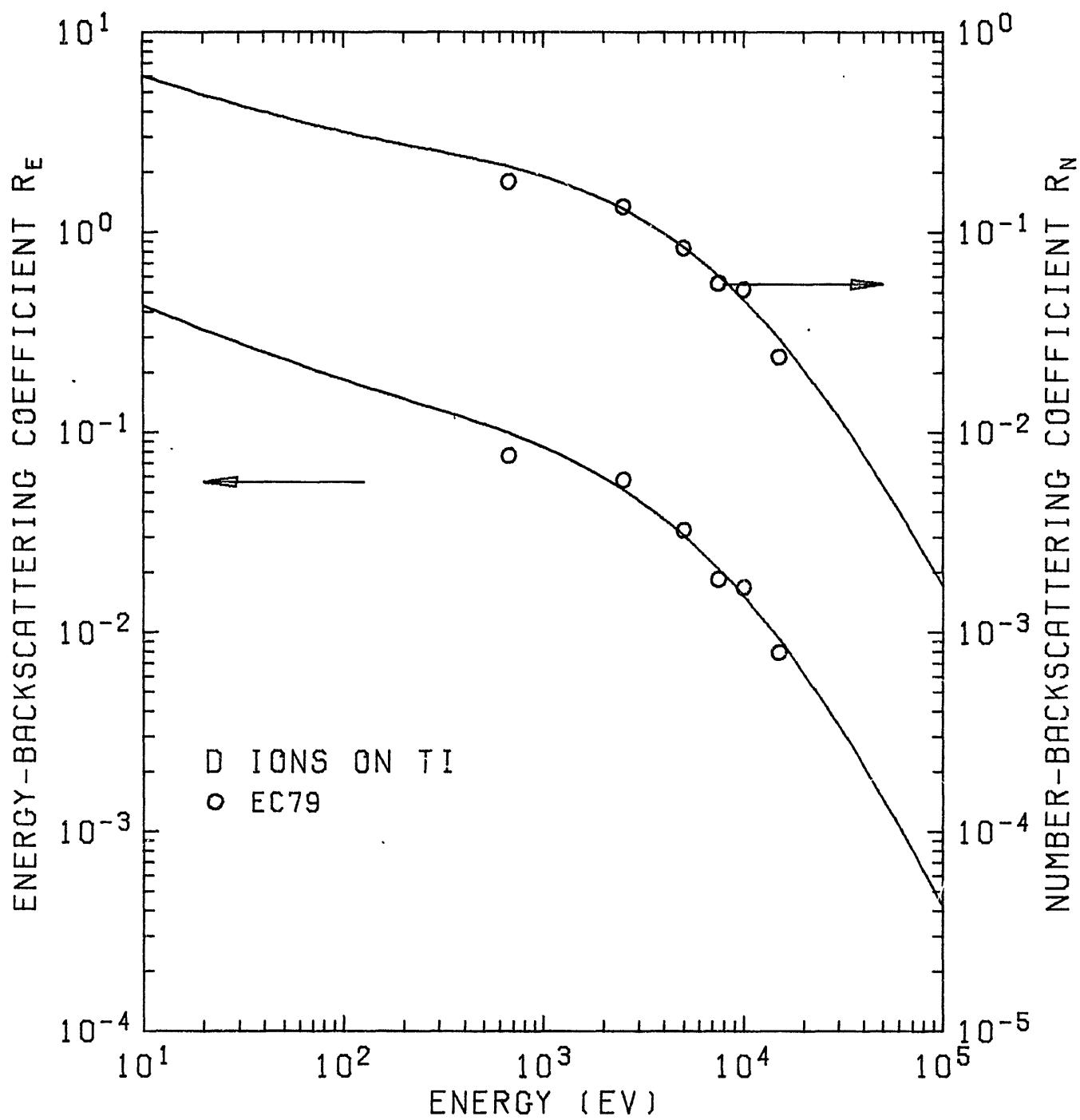
Fig. 17.  $R_N$  and  $R_E$  of D ions on  $^{22}\text{Ti}$ .
