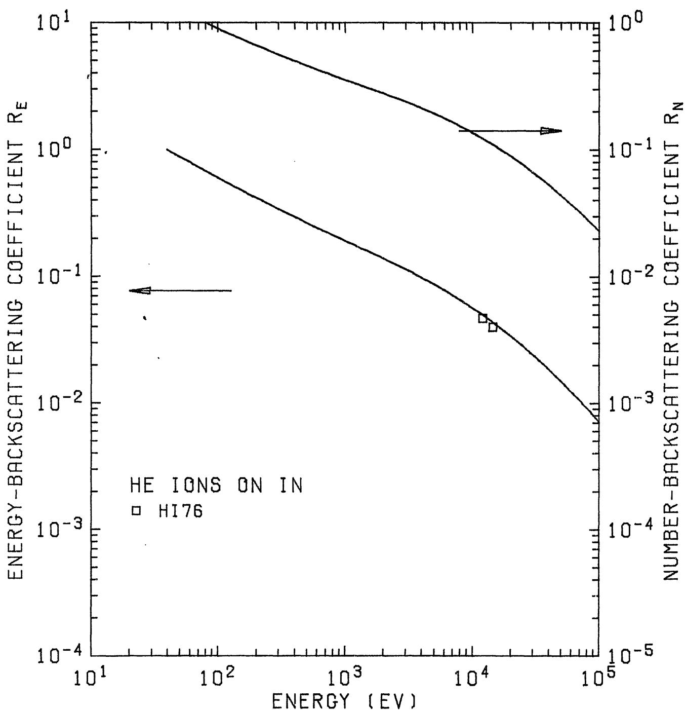
Fig. 46.  $R_N$  and  $R_E$  of He ions on  $_{49}\text{In}$ .
