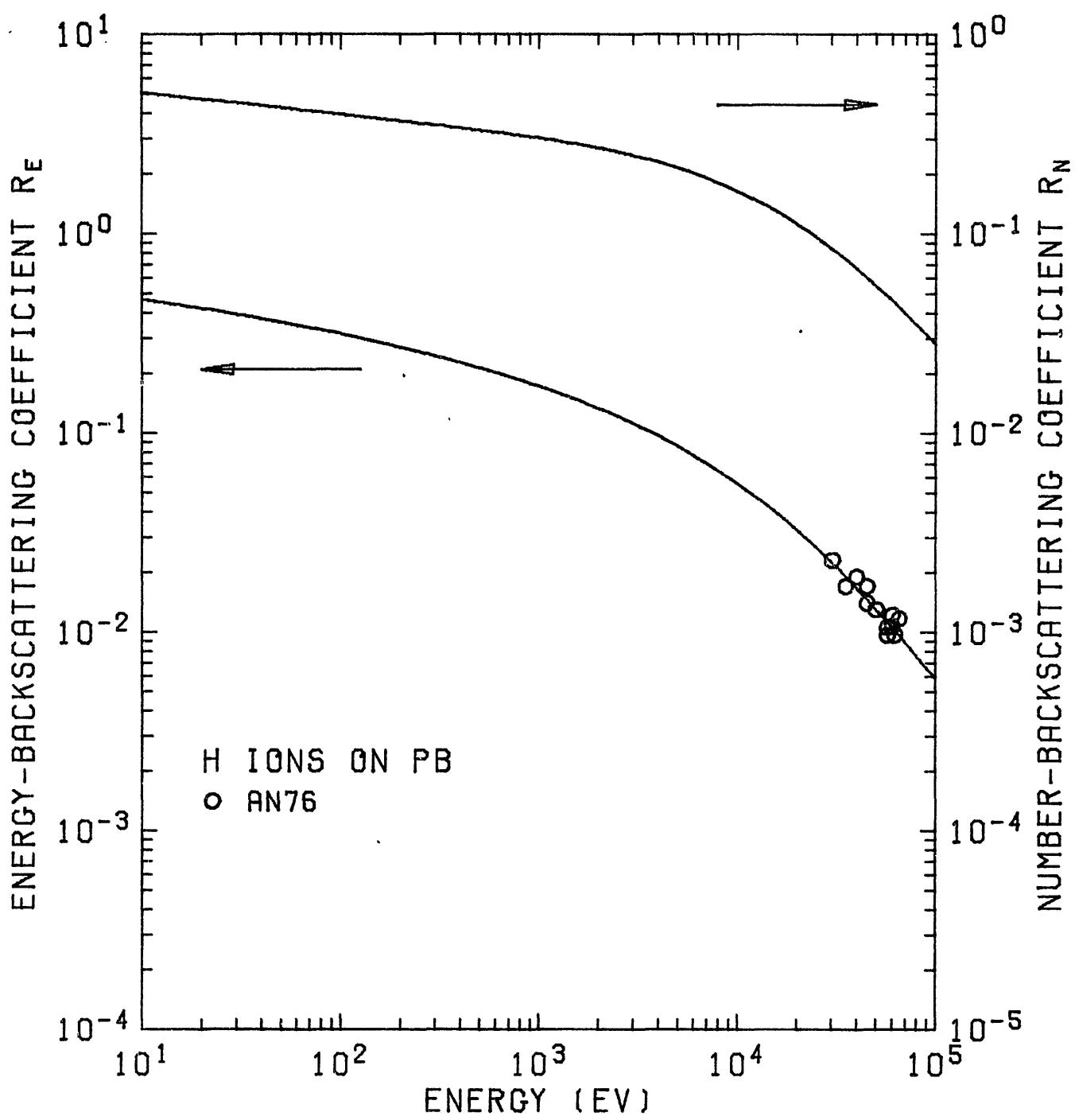
Fig. 15.  $R_N$  and  $R_E$  of H ions on  $^{82}\text{Pb}$ .
