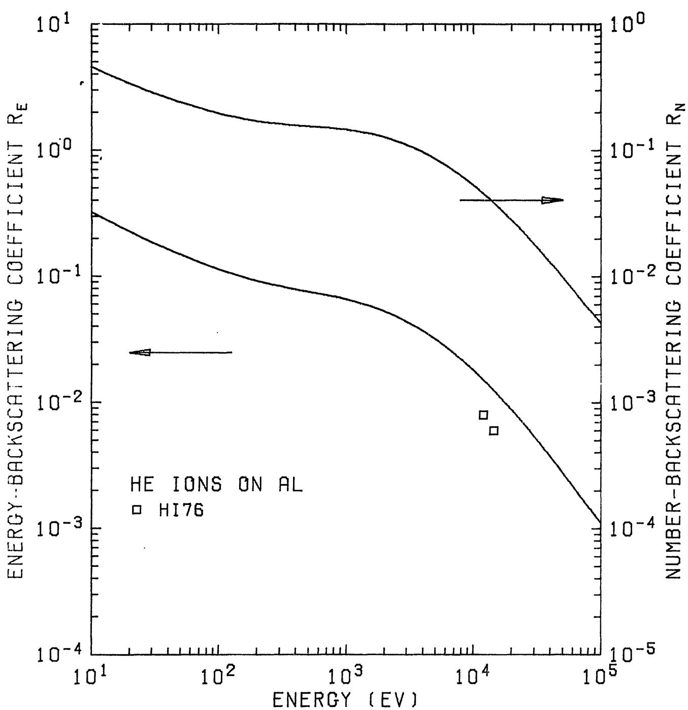
Fig. 26.  $R_N$  and  $R_E$  of He ions on  $^{13}\text{Al}$ .
