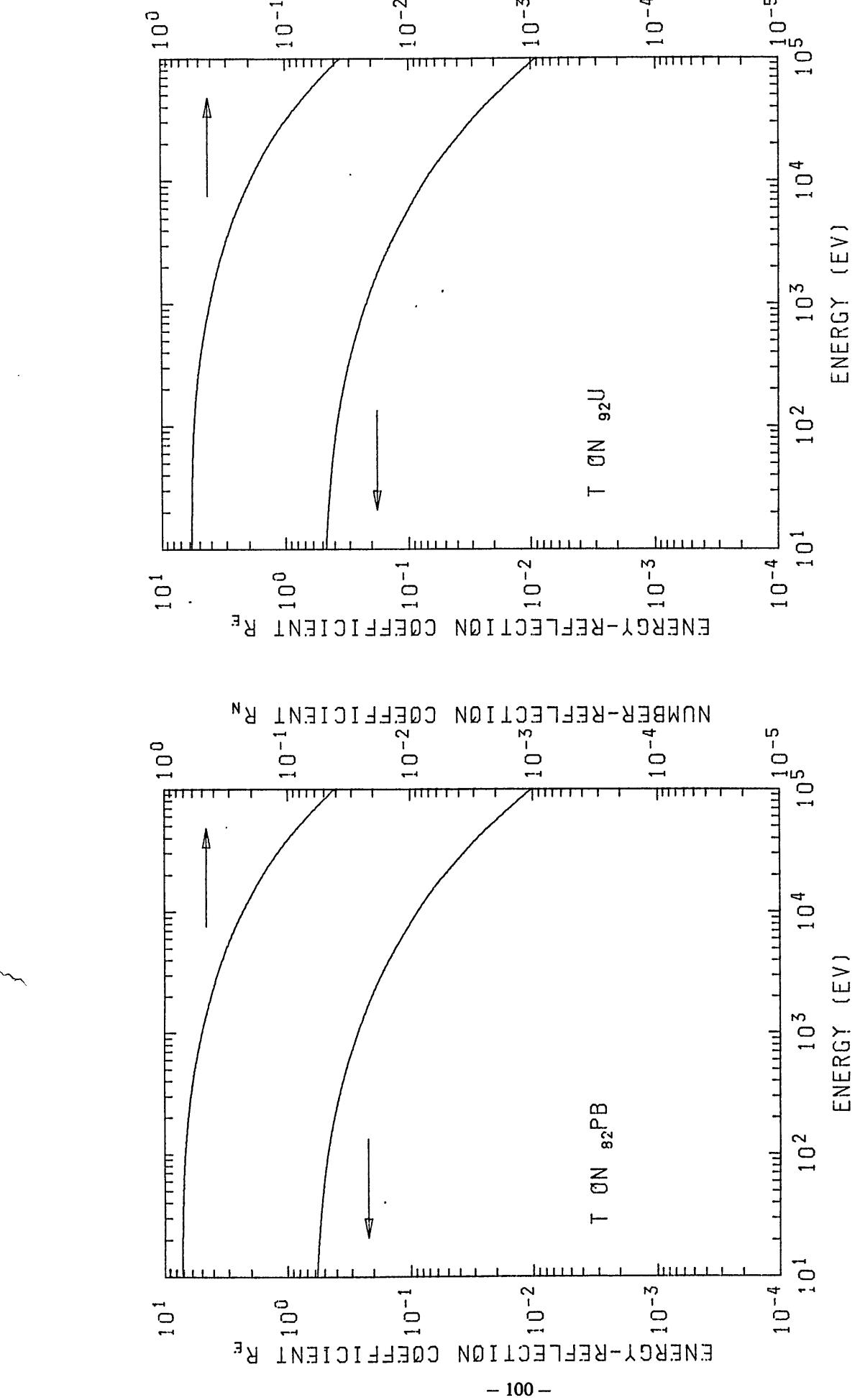
GRAPH III.  $R_N$  and  $R_E$  vs Energy for T Ions on Pb and U
